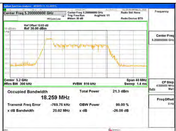
MID CHANNEL OBW
