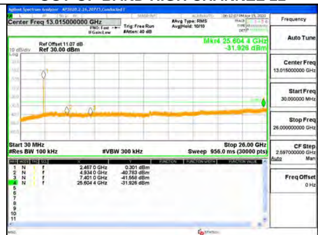
OUT-OF-BAND HIGH CHANNEL 11
