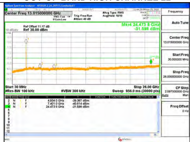
OUT-OF-BAND HIGH CHANNEL 11
