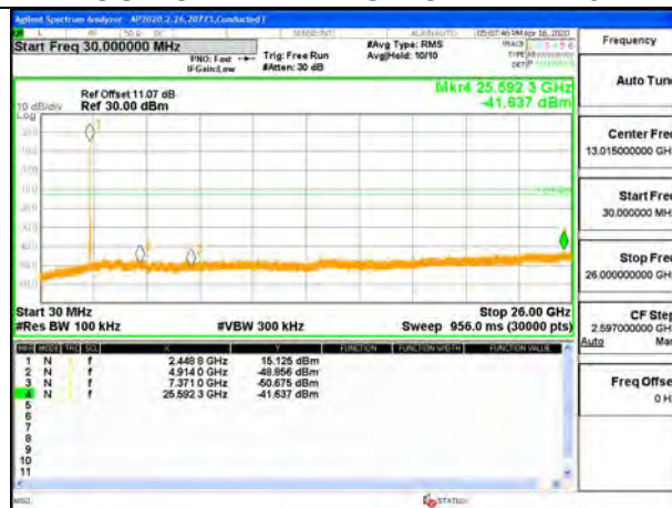
OUT-OF-BAND HIGH CHANNEL 9
