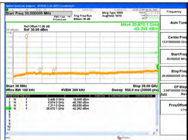
OUT-OF-BAND MID CHANNEL
