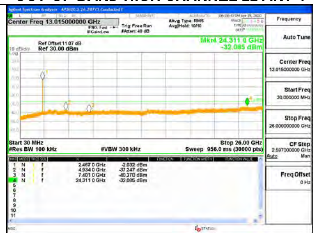
OUT-OF-BAND HIGH CHANNEL 11 ANT 4
