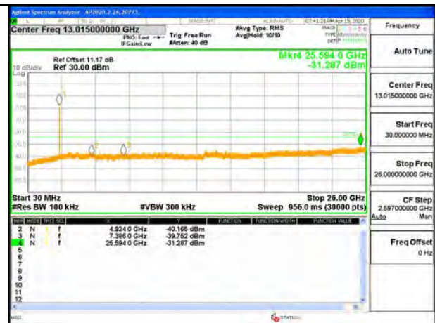
OUT-OF-BAND HIGH CHANNEL 11
