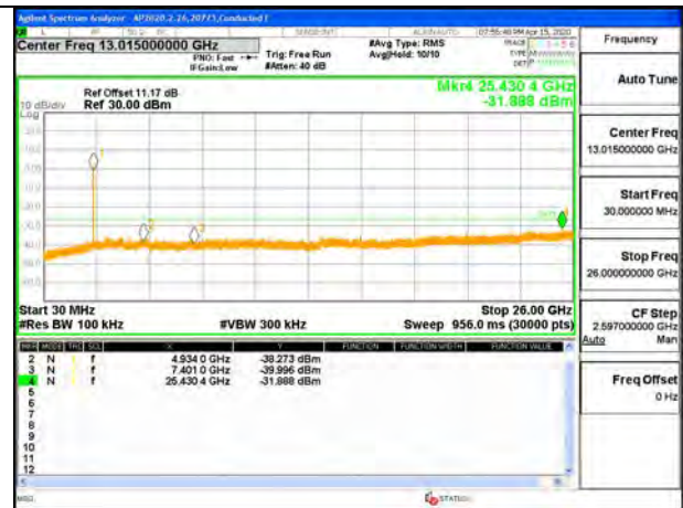
OUT-OF-BAND HIGH CHANNEL 11 ANT 3
