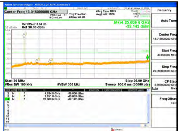
OUT-OF-BAND LOW CHANNEL 1
