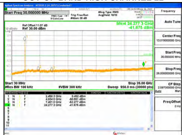
OUT-OF-BAND HIGH CHANNEL 11
