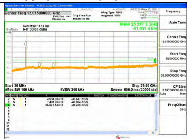
OUT-OF-BAND HIGH CHANNEL 11
