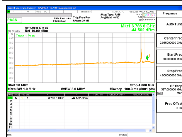
LTE B48 20MHz QPSK Mid Channel RB1-0 (30MHz to 4GHz)
