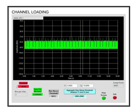
The level of traffic loading on the channel by the EUT is 20.05%
