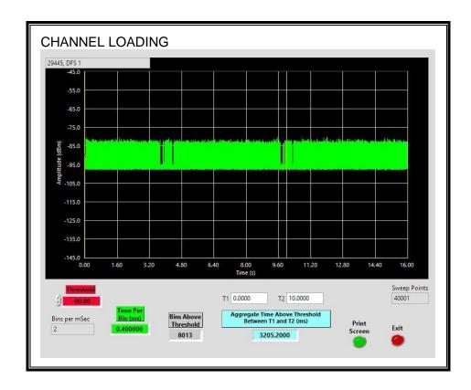
The level of traffic loading on the channel by the EUT is 32.05%
