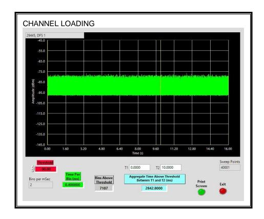
The level of traffic loading on the channel by the EUT is 28.42%
