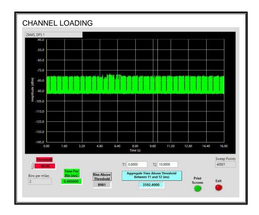
The level of traffic loading on the channel by the EUT is 35.92%
