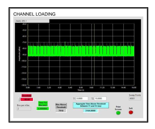
The level of traffic loading on the channel by the Peer Slave is 31.64%
