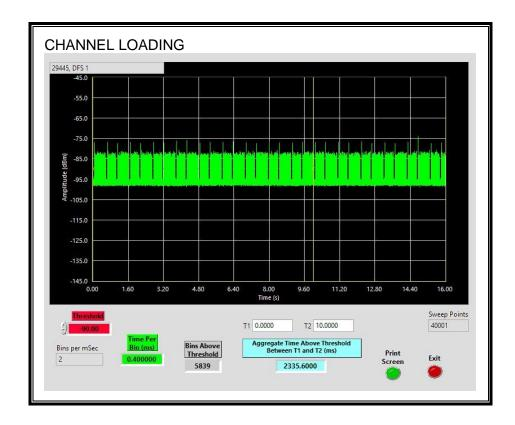
The level of traffic loading on the channel by the Peer Slave is 23.35%
