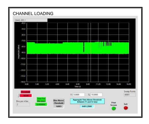
The level of traffic loading on the channel by the EUT is 64.01%
