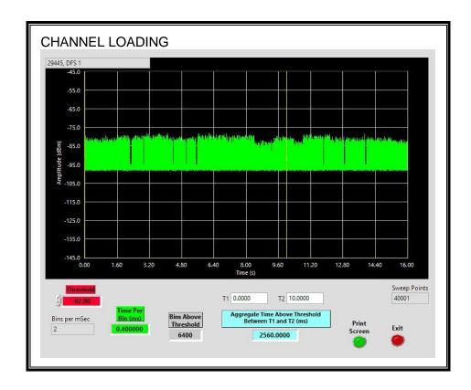
The level of traffic loading on the channel by the EUT is 25.6%
