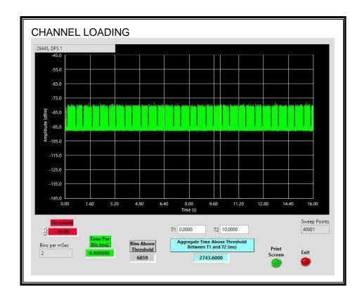
The level of traffic loading on the channel by the EUT is 27.43%
