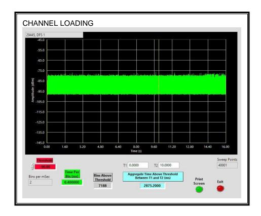
The level of traffic loading on the channel by the EUT is 28.75%
