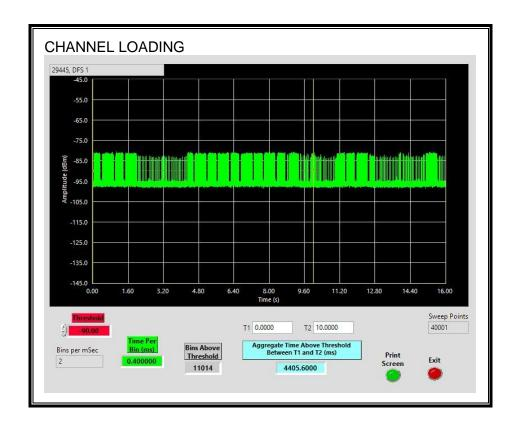
The level of traffic loading on the channel by the EUT is 44.05%
