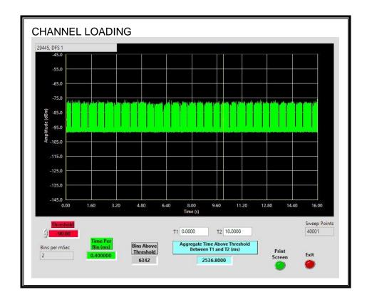
The level of traffic loading on the channel by the EUT is 25.36%
