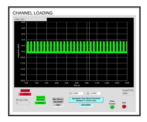
The level of traffic loading on the channel by the Peer Slave is 29.2%
