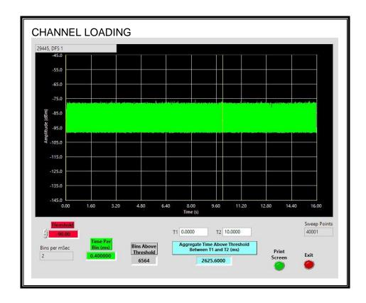
The level of traffic loading on the channel by the EUT is 26.25%
