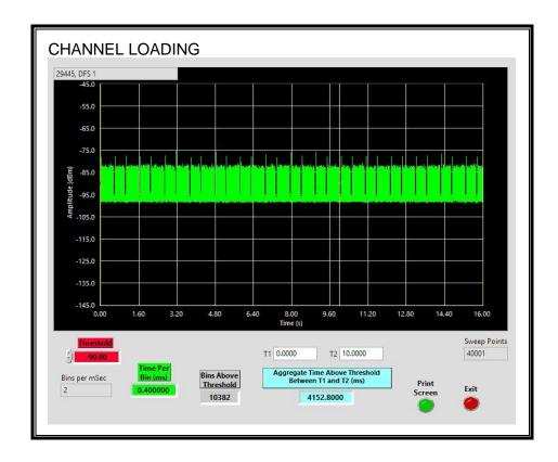
The level of traffic loading on the channel by the Peer Slave is 41.52%
