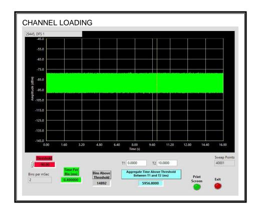
The level of traffic loading on the channel by the EUT is 59.56%
