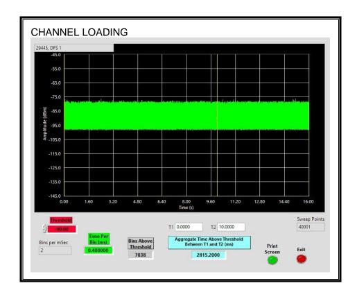
The level of traffic loading on the channel by the EUT is 28.15%
