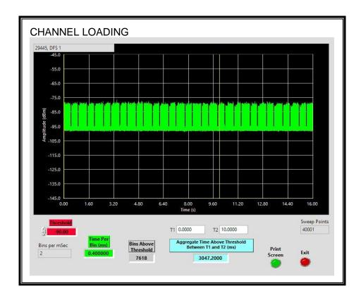
The level of traffic loading on the channel by the EUT is 30.47%
