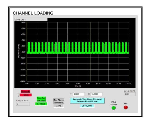
The level of traffic loading on the channel by the Peer Slave is 29.49%
