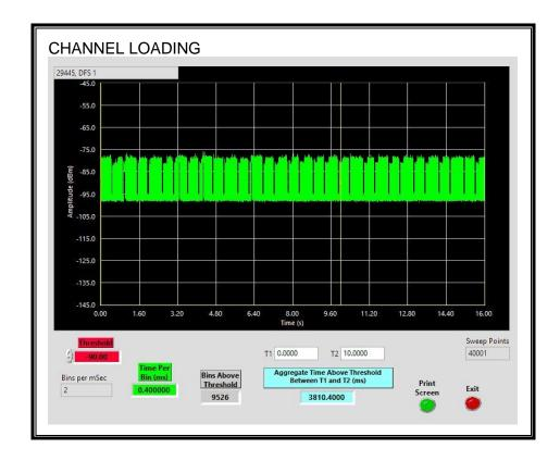
The level of traffic loading on the channel by the EUT is 38.1%
