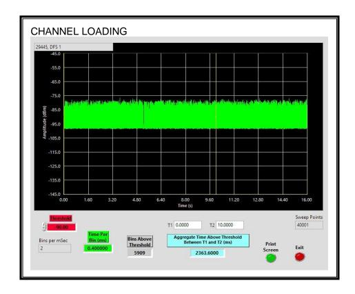
The level of traffic loading on the channel by the EUT is 23.63%
