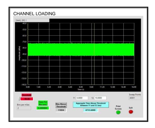
The level of traffic loading on the channel by the EUT is 47.33%
