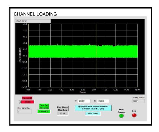
The level of traffic loading on the channel by the EUT is 29.34%
