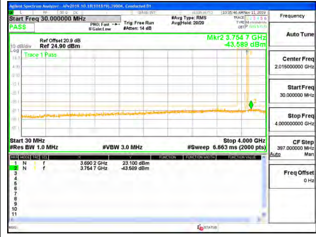
LTE B48 10MHz 16QAM High Channel RB1-0 (30MHz to 4GHz)
