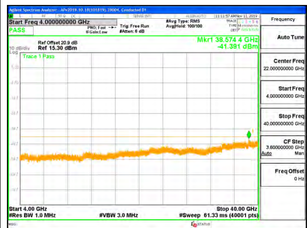
LTE B48 5MHz 16QAM High Channel RB1-0 (4G to 40G)
