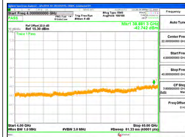
LTE B48 15MHz QPSK High Channel RB1-0 (4G to 40G)
