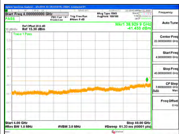
LTE B48 10MHz 16QAM High Channel RB1-0 (4G to 40G)
