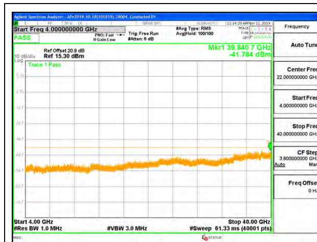
LTE B48 10MHz QPSK Middle Channel RB1-0 (4G to 40G)
