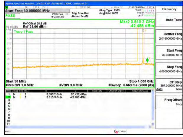
LTE B48 15MHz 16QAM High Channel RB1-0 (30MHz to 4GHz)
