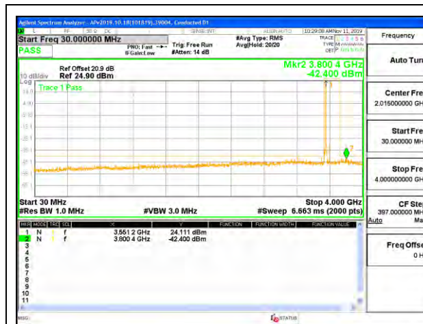
LTE B48 10MHz QPSK Low Channel RB1-0 (30MHz to 4GHz)
