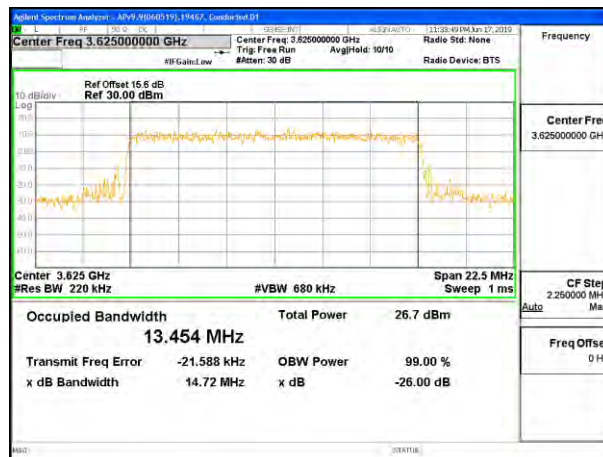
LTE B48 15MHz 64QAM Middle Channel RB75-0
