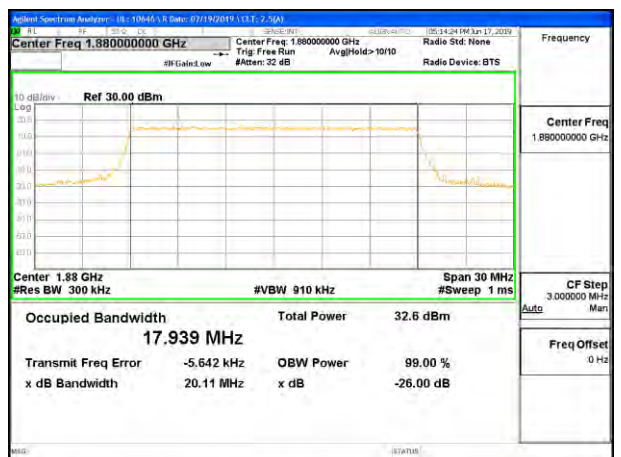
LTE B2 20MHz 64QAM Middle Channel RB100-0
