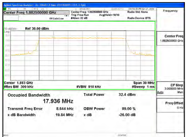
LTE B25 20MHz 64QAM Middle Channel RB100-0
