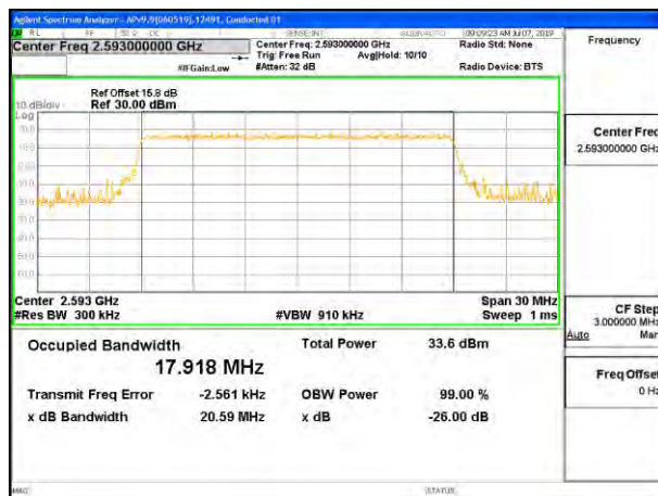
LTE B41 20MHz 16QAM Middle Channel RB100-0
