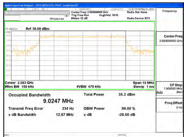
LTE B41 10MHz QPSK Middle Channel RB50-0
