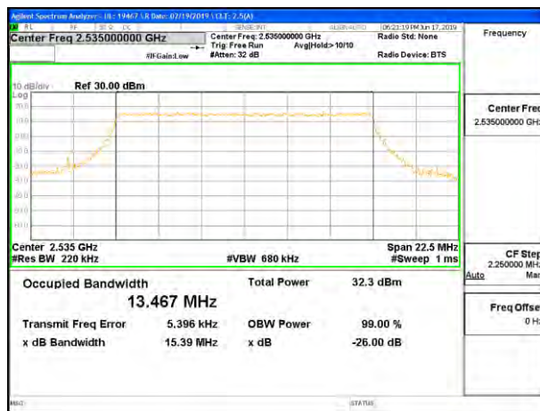
LTE B7 15MHz 64QAM Middle Channel RB75-0
