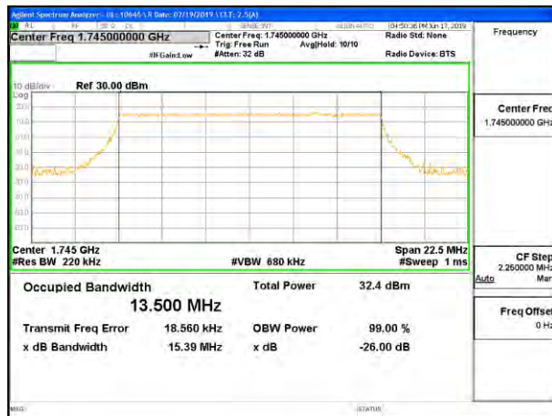
LTE B66 15MHz 64QAM Middle Channel RB75-0
