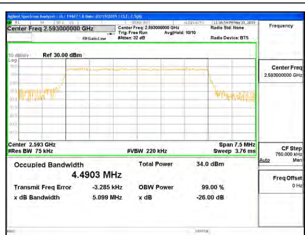
LTE B41 5MHz 16QAM Middle Channel RB25-0
