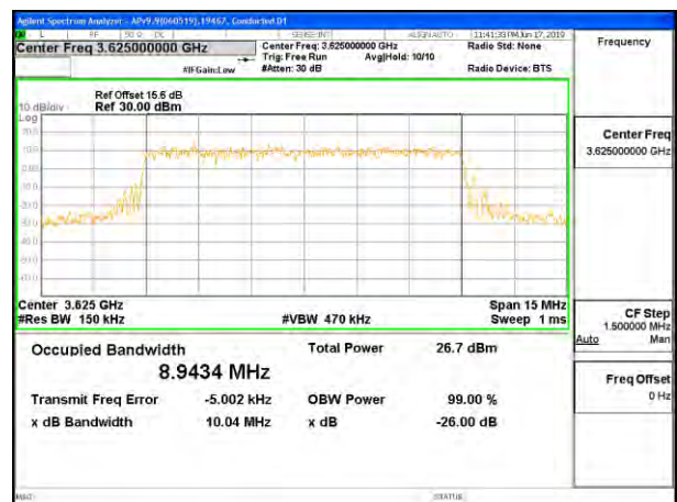
LTE B48 10MHz 64QAM Middle Channel RB50-0
