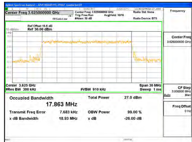
LTE B48 20MHz 64QAM Middle Channel RB100-0
