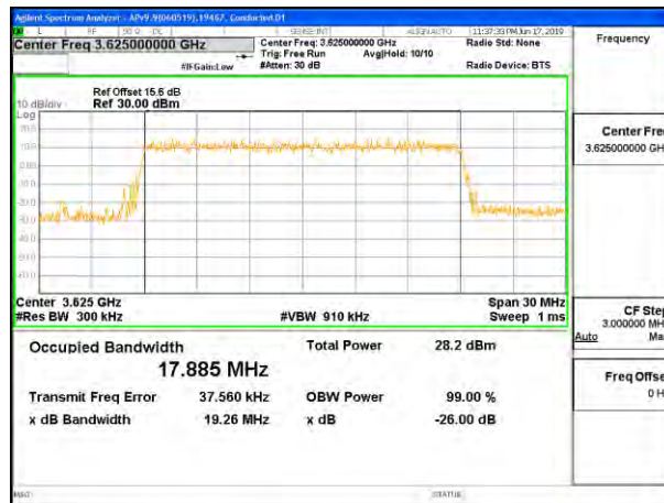
LTE B48 20MHz 16QAM Middle Channel RB100-0
