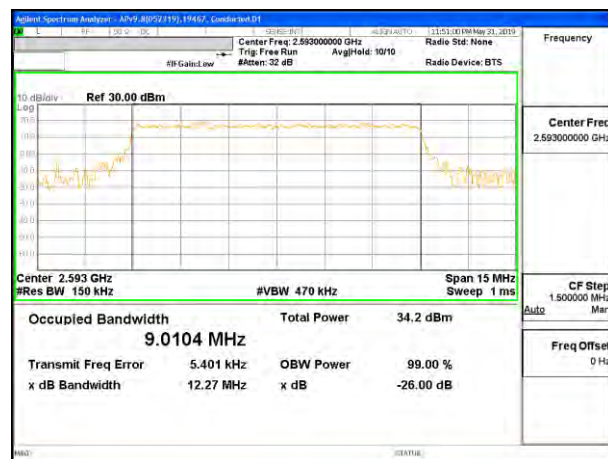
LTE B41 10MHz 16QAM Middle Channel RB50-0
