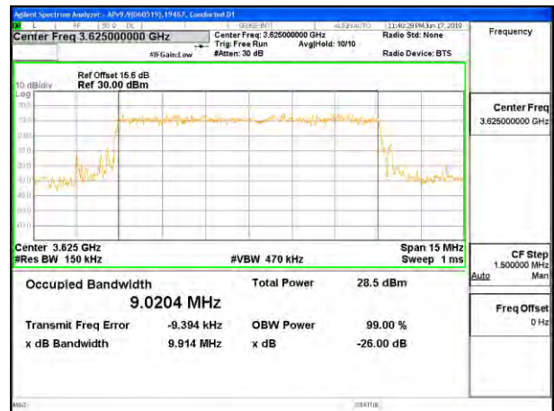
LTE B48 10MHz QPSK Middle Channel RB50-0
