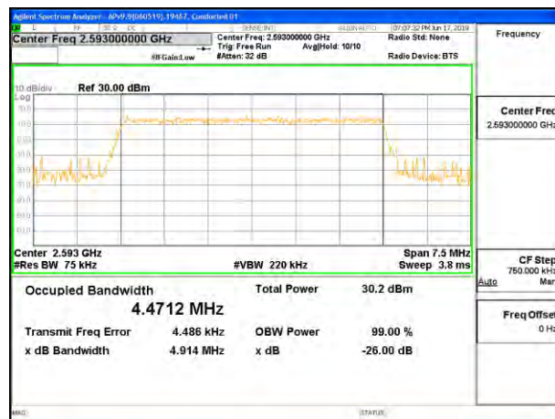
LTE B41 5MHz 64QAM Middle Channel RB25-0
