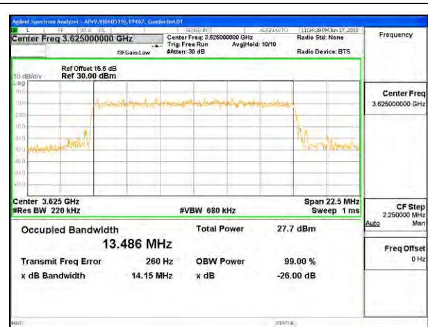
LTE B48 15MHz 16QAM Middle Channel RB75-0
