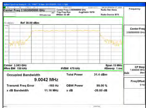
LTE B41 10MHz 64QAM Middle Channel RB50-0
