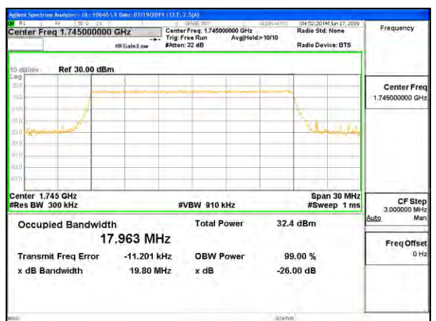
LTE B66 20MHz 64QAM Middle Channel RB100-0
