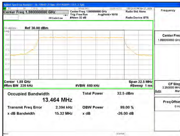
LTE B2 15MHz 64QAM Middle Channel RB75-0
