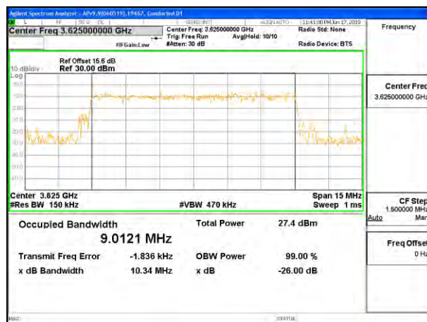
LTE B48 10MHz 16QAM Middle Channel RB50-0
