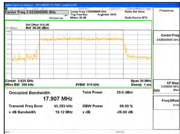
LTE B48 20MHz QPSK Middle Channel RB100-0
