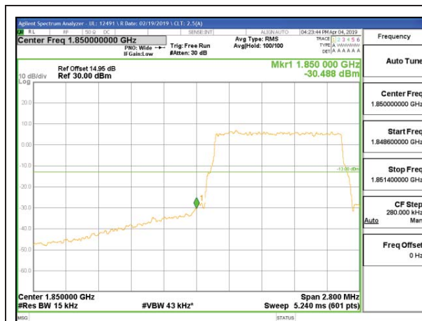
LTE B25 1.4MHz 16QAM Low Channel RB6-0
