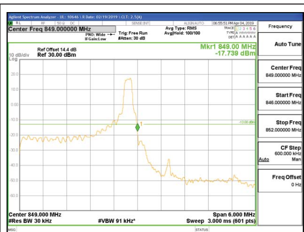
LTE B5 3MHz 16QAM High Channel RB1-14
