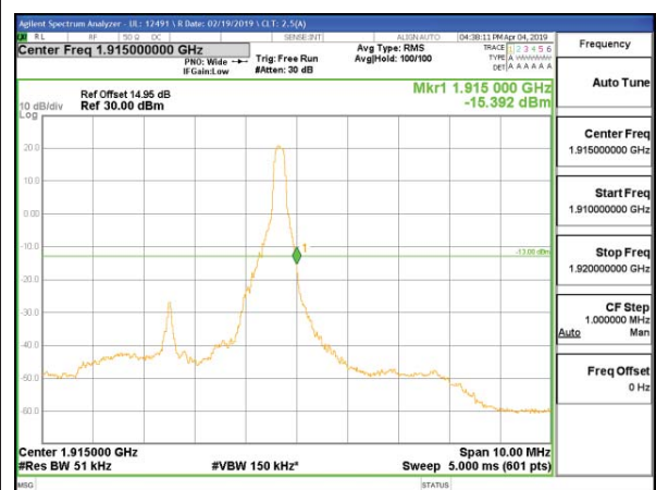
LTE B25 5MHz QPSK High Channel RB1-24
