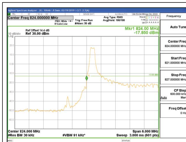
LTE B5 3MHz 16QAM Low Channel RB1-0
