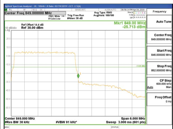
LTE B5 3MHz 16QAM High Channel RB15-0
