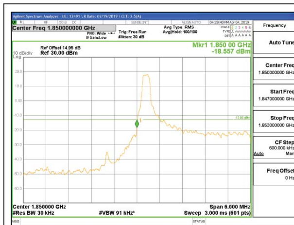
LTE B25 3MHz 16QAM Low Channel RB1-0
