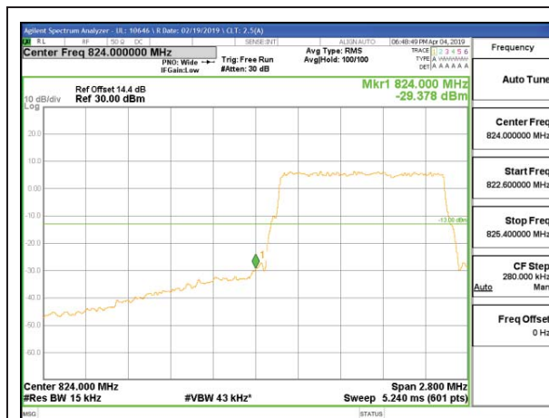
LTE B5 1.4MHz 16QAM Low Channel RB6-0
