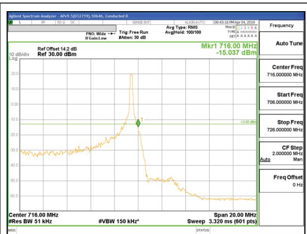
LTE B17 10MHz 16QAM High Channel RB1-9
