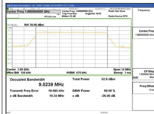
LTE B2 10MHz 16QAM Middle Channel RB50-0
