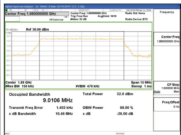
LTE B2 10MHz 64QAM Middle Channel RB50-0
