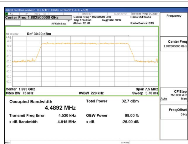
LTE B25 5MHz 16QAM Middle Channel RB25-0
