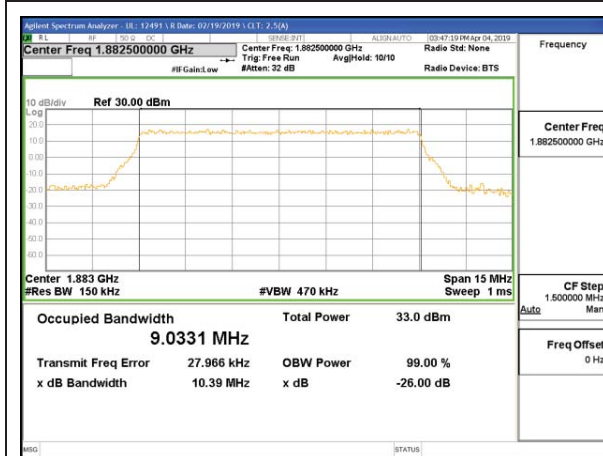
LTE B25 10MHz 16QAM Middle Channel RB50-0
