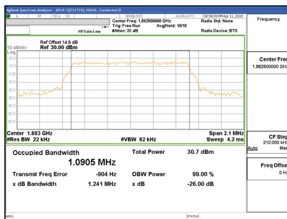
LTE B25 1.4MHz 64QAM Middle Channel RB6-0
