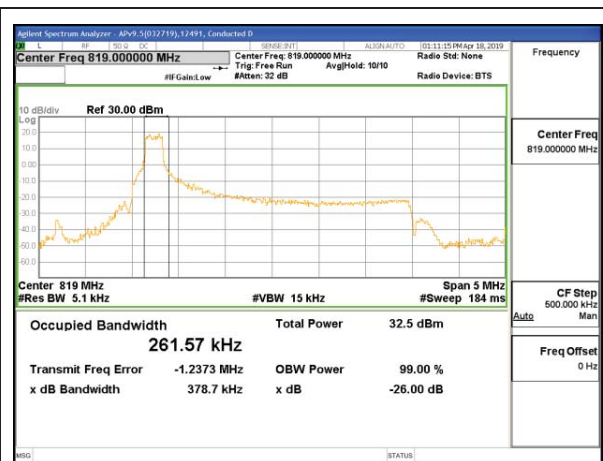
LTE B26 3MHz 16QAM Middle Channel RB1-0
