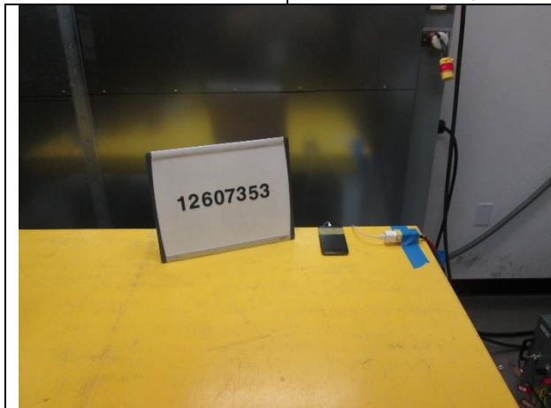
AC LINE CONDUCTED (FRONT)
