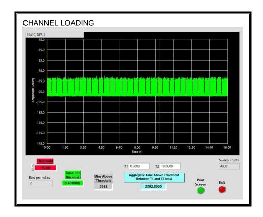
The level of traffic loading on the channel by the EUT is 23.92%
