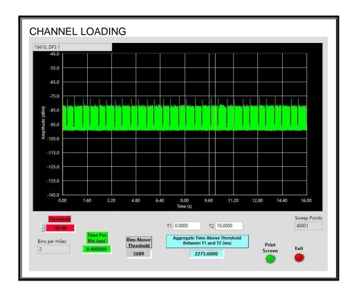
The level of traffic loading on the channel by the Peer Slave is 22.75%
