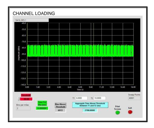
The level of traffic loading on the channel by the EUT is 27.88%
