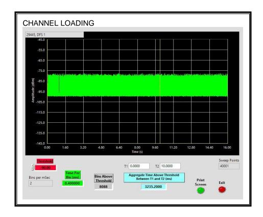
The level of traffic loading on the channel by the EUT is 32.35%
