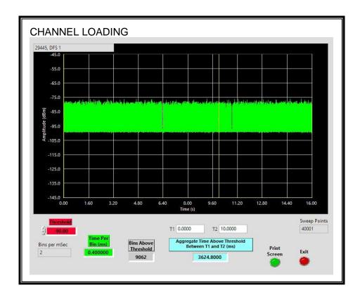
The level of traffic loading on the channel by the EUT is 36.24%
