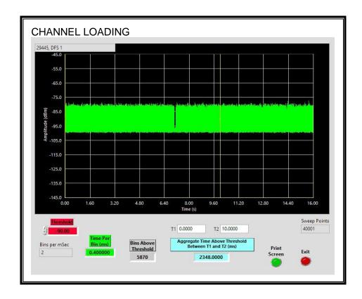
The level of traffic loading on the channel by the EUT is 23.48%
