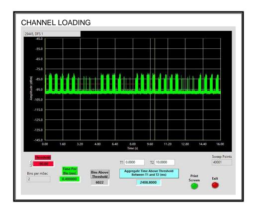
The level of traffic loading on the channel by the EUT is 24.08%
