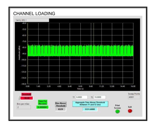
The level of traffic loading on the channel by the EUT is 33.31%
