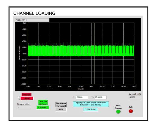
The level of traffic loading on the channel by the Peer Slave is 27.01%
