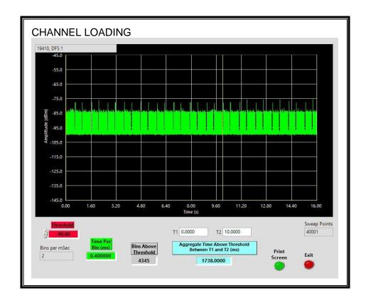
The level of traffic loading on the channel by the Peer Slave is 17.38%
