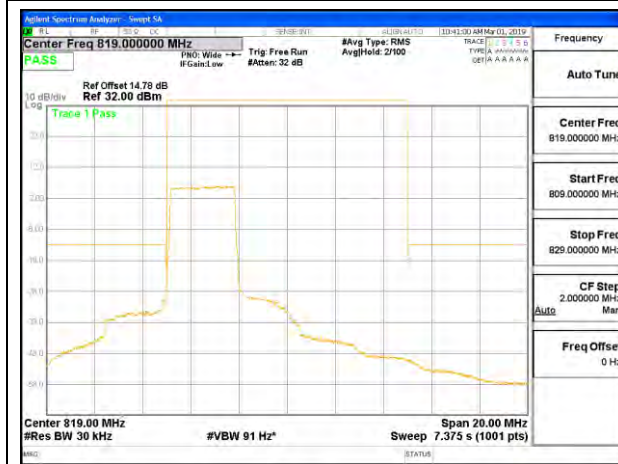
LTE B26 3MHz QPSK Low Channel RB15-0 ID:12491
