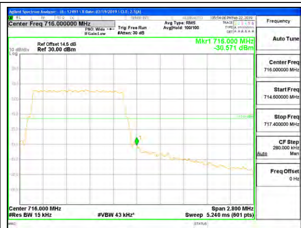
LTE B12 1.4MHz 16QAM High Channel RB6-0
