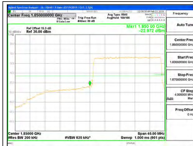
LTE B25 20MHz QPSK Low Channel RB100-0
