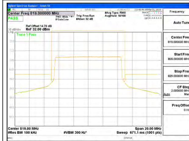
LTE B26 10MHz QPSK Middle Channel RB50-0 ID:12491
