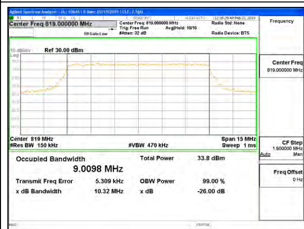
LTE B26 10MHz QPSK Middle Channel RB50-0
