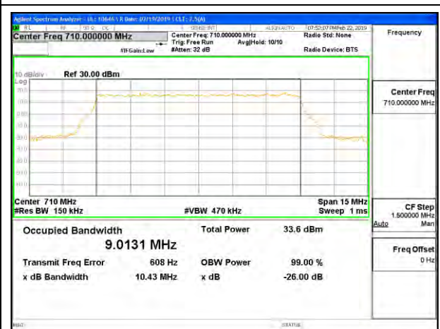
LTE B17 10MHz QPSK Middle Channel RB50-0
