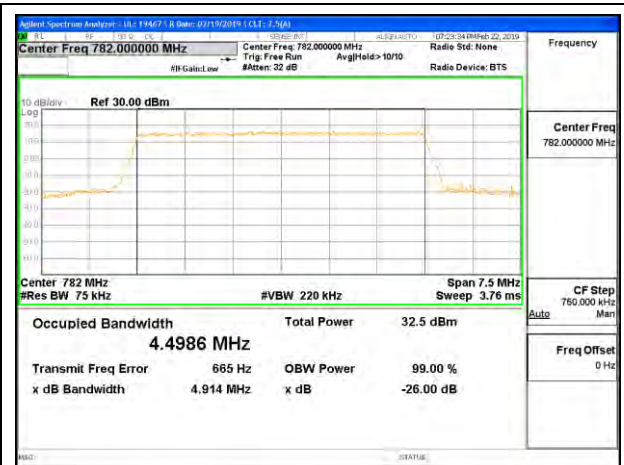
LTE B13 5MHz 16QAM Middle Channel RB25-0
