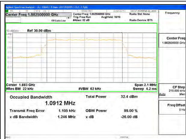
LTE B25 1.4MHz 16QAM Middle Channel RB6-0
