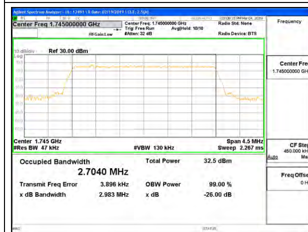
LTE B66 3MHz 16QAM Middle Channel RB15-0
