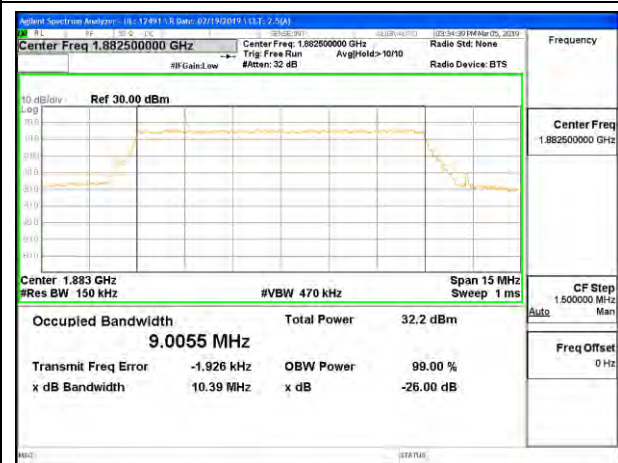
LTE B25 10MHz 64QAM Middle Channel RB50-0
