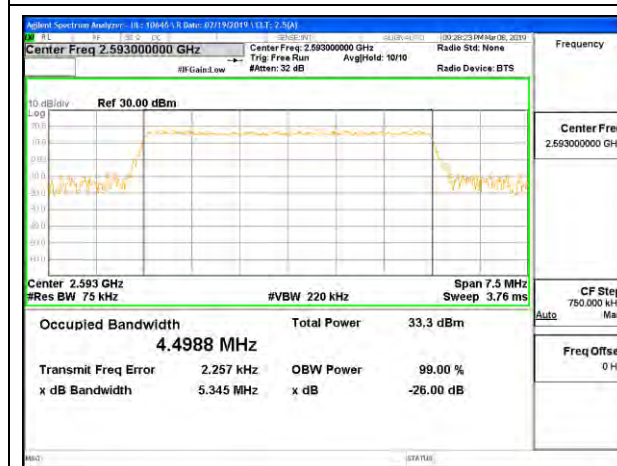
LTE B41 5MHz 64QAM Middle Channel RB25-0
