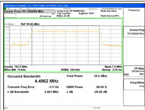
LTE B12 5MHz 16QAM Middle Channel RB25-0
