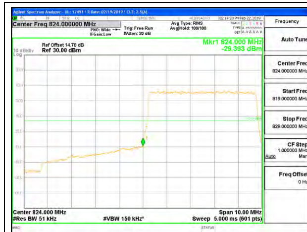
LTE B5 5MHz QPSK Low Channel RB25-0
