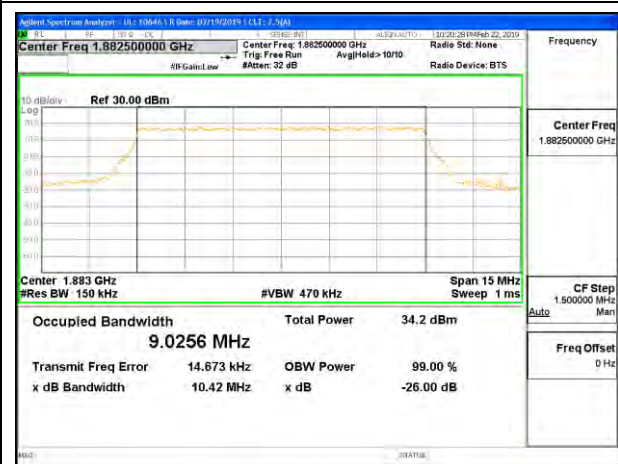
LTE B25 10MHz QPSK Middle Channel RB50-0
