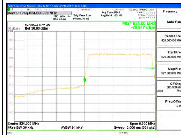
LTE B5 3MHz 16QAM Low Channel RB15-0
