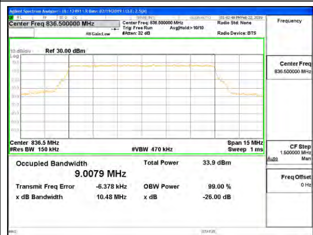
LTE B5 10MHz QPSK Middle Channel RB50-0
