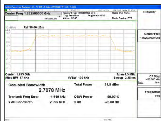
LTE B25 3MHz 64QAM Middle Channel RB15-0
