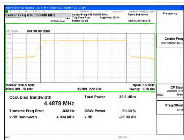
LTE B5 5MHz 16QAM Middle Channel RB25-0
