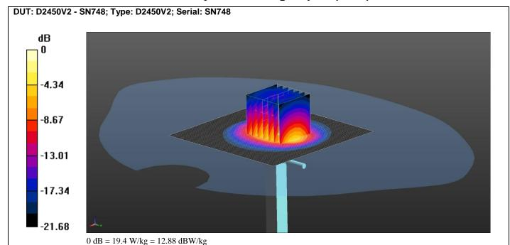
Communication System: UID 0, CW (0); Frequency: 2450 MHz; Duty Cycle: 1:1 Medium: 2450 MSL Medium parameters used: f = 2450 MHz;  $\sigma = 2.02$  S/m;  $\epsilon_r = 50.632$ ;  $\rho = 1000$  kg/m<sup>3</sup>
