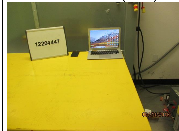
AC LINE CONDUCTED WITH LAPTOP (FRONT)
