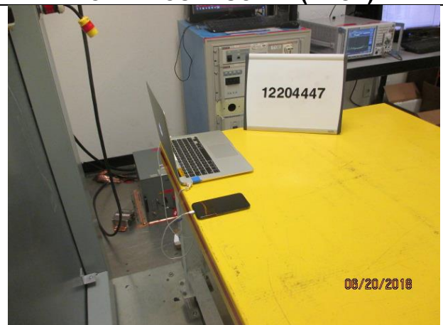
AC LINE CONDUCTED WITH LAPTOP (BACK)
