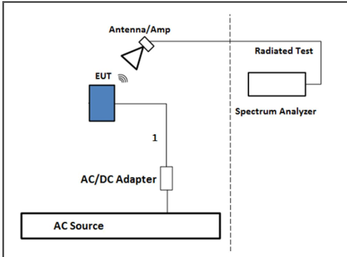
**TEST SETUP- AC LINE CONDUCTED: AC/DC ADAPTER**
