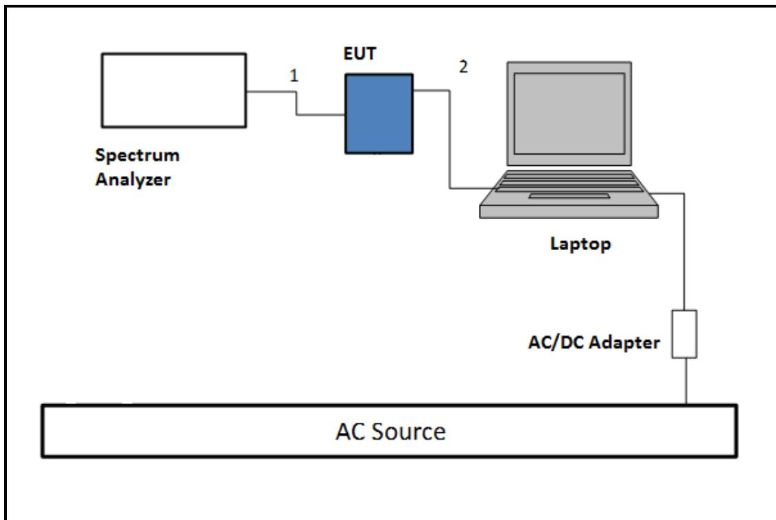
**TEST SETUP- RADIATED-ABOVE 1 GHZ**
