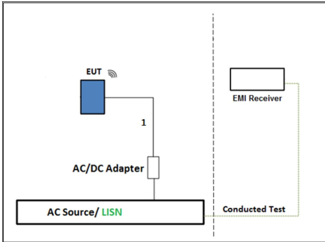
**TEST SETUP- AC LINE CONDUCTED: LAPTOP CONFIGURATION**
