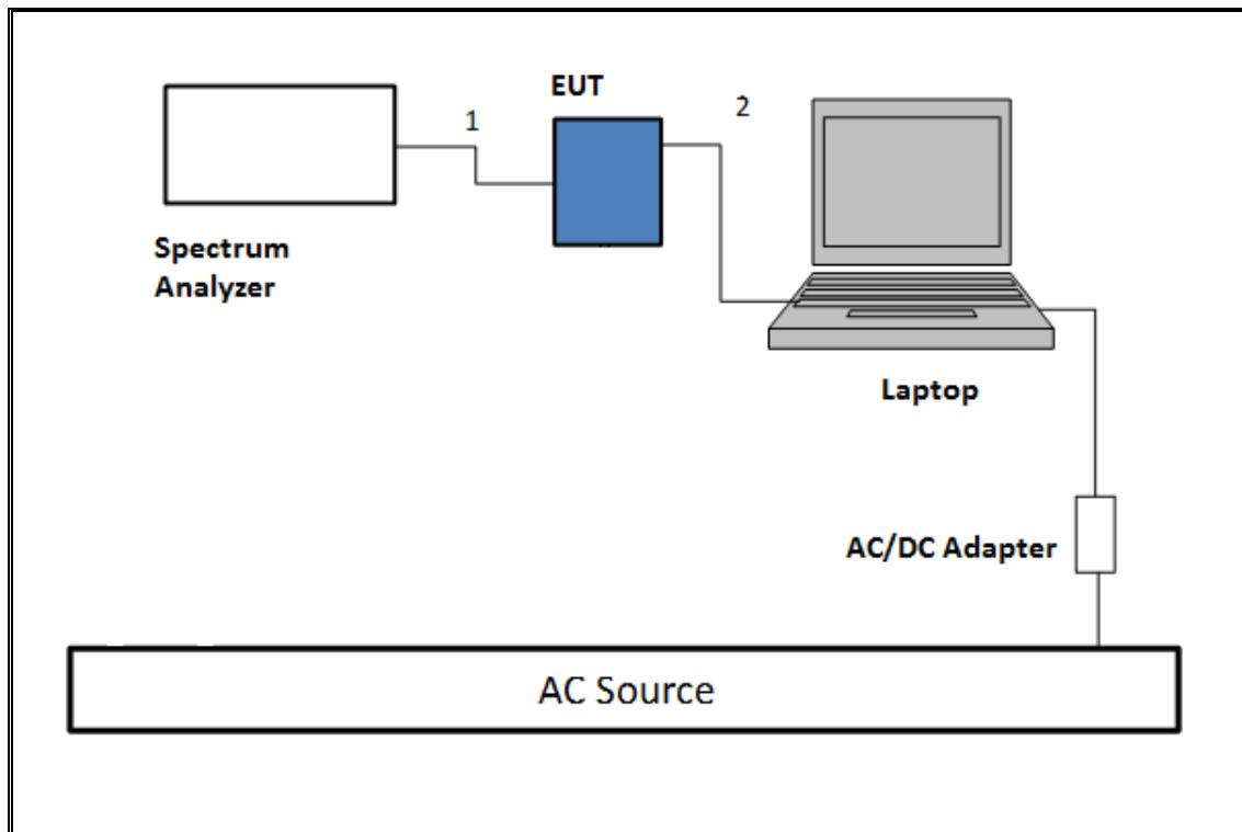
**TEST SETUP- RADIATED-ABOVE 1 GHZ**
