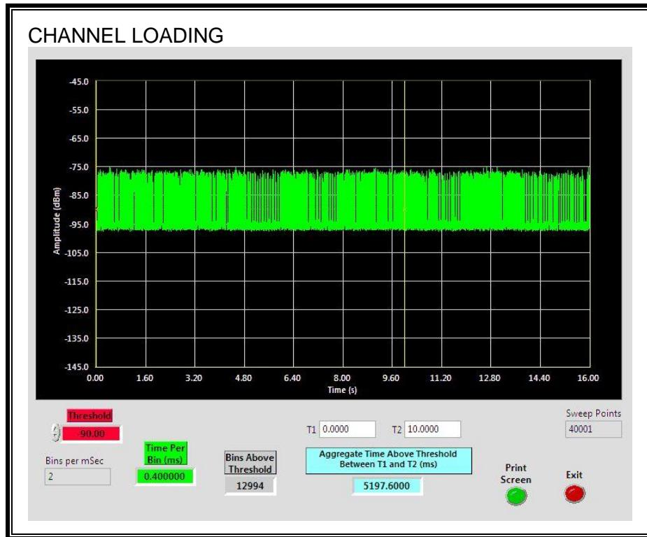
The level of traffic loading on the channel by the EUT is 51.97%
