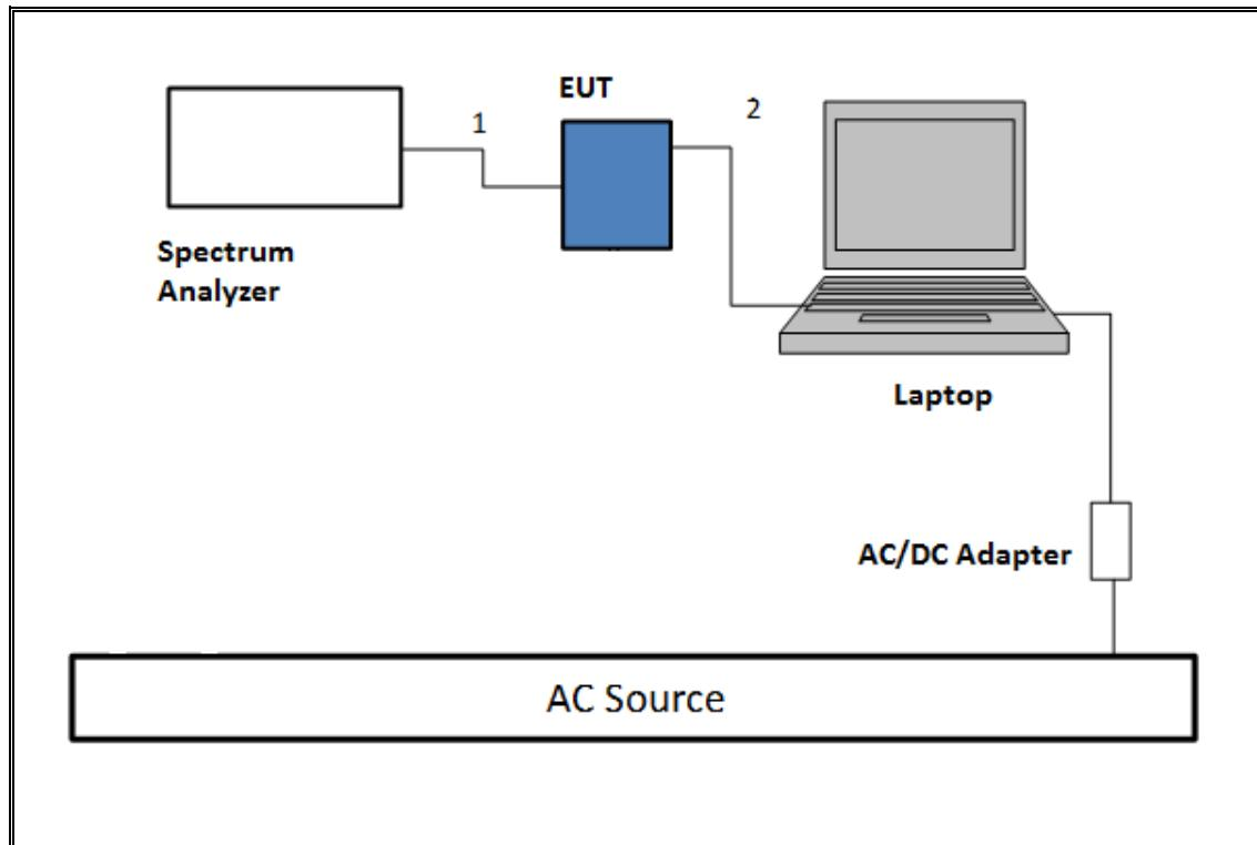
**TEST SETUP- RADIATED-ABOVE 1 GHZ**
