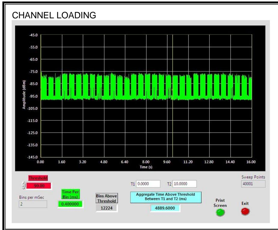
The level of traffic loading on the channel by the EUT is 48.89%
