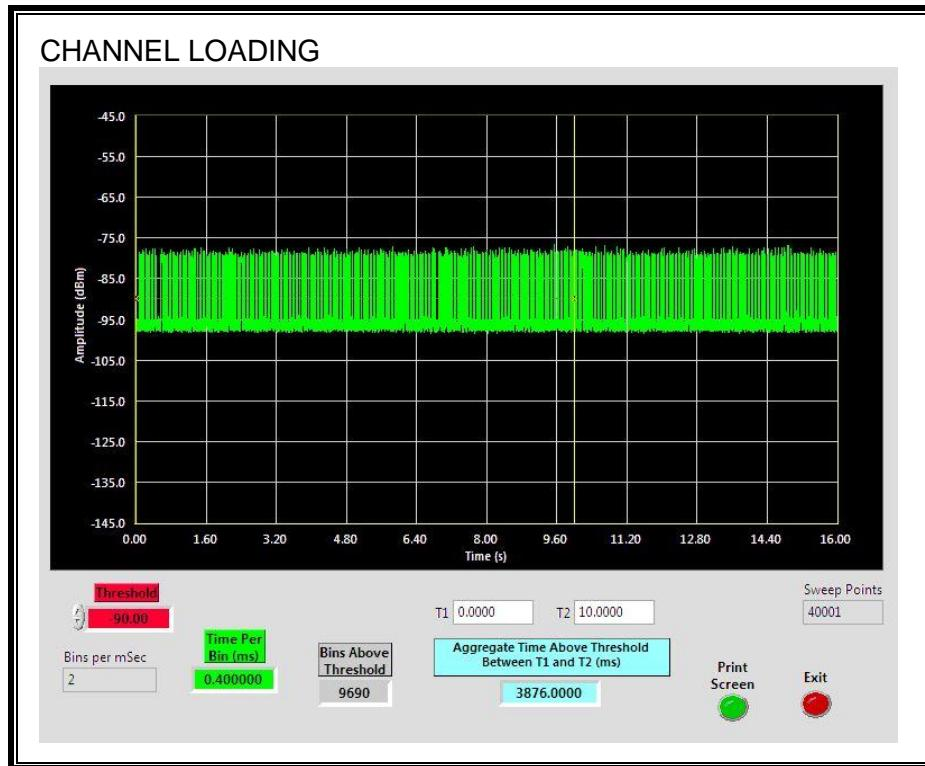
The level of traffic loading on the channel by the EUT is 38.76%
