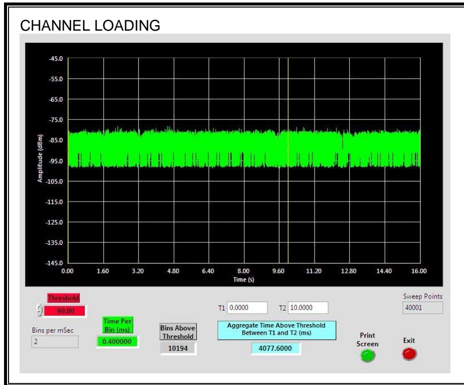
The level of traffic loading on the channel by the EUT is 40.77%
