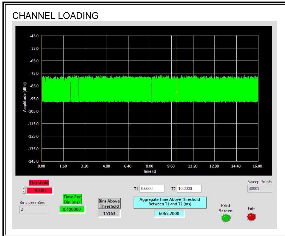
The level of traffic loading on the channel by the EUT is 60.65%
