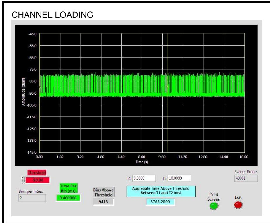
The level of traffic loading on the channel by the EUT is 37.65%
