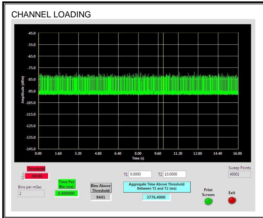
The level of traffic loading on the channel by the EUT is 37.76%
