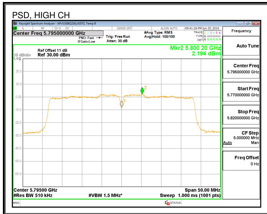
**7.54. 802.11n HT40 2Tx STBC MODE IN THE 5.8 GHz BAND****Note:** Covered by 802.11n HT40 2Tx CDD MODE
