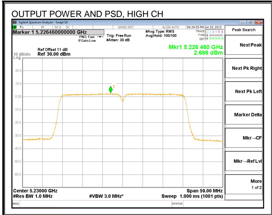
**8.8. 802.11n HT40 2Tx STBC MODE IN THE 5.2 GHz BAND****Note:** Covered by 802.11n HT40 2Tx CDD MODE
