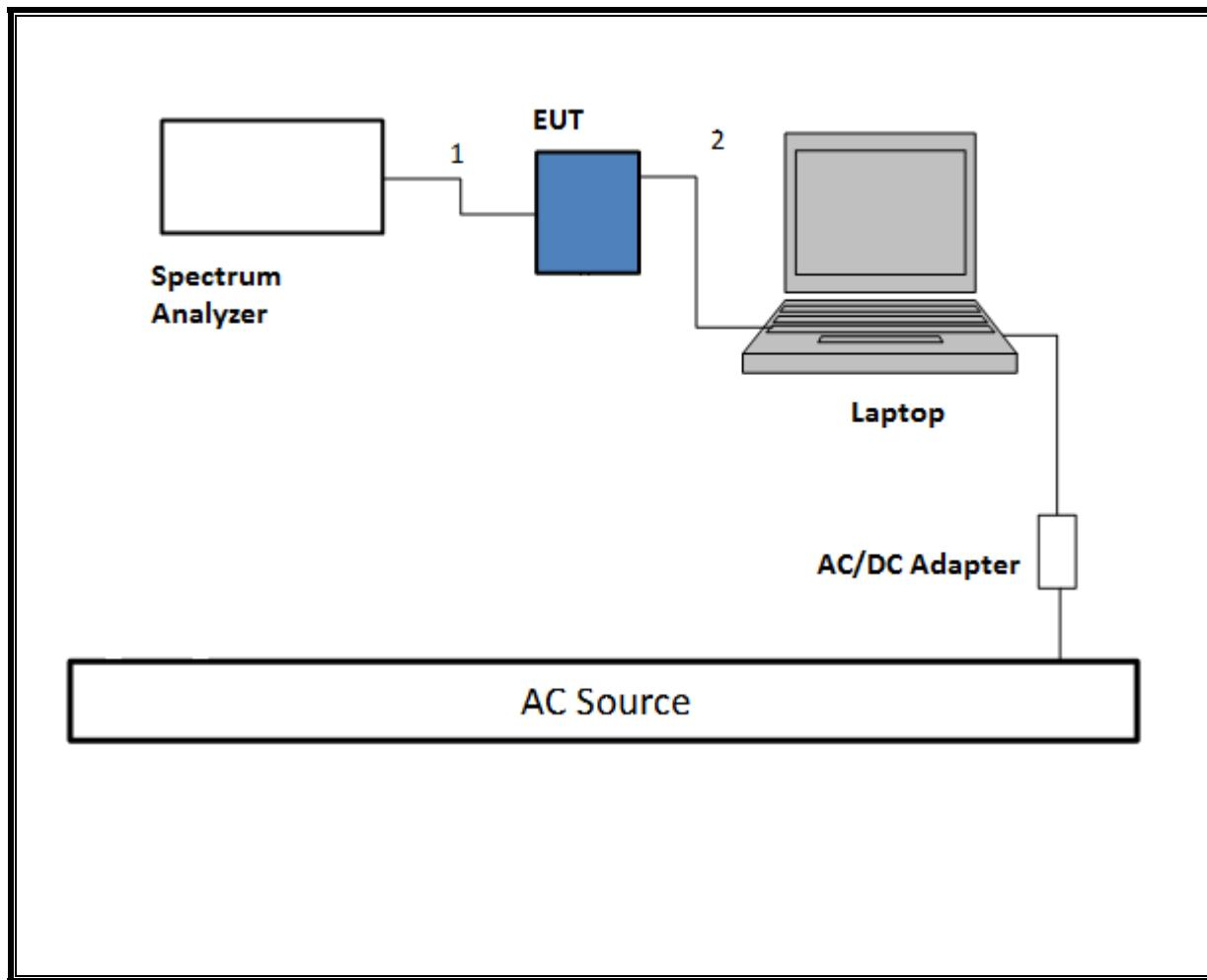
**TEST SETUP- RADIATED-ABOVE 1 GHZ**
