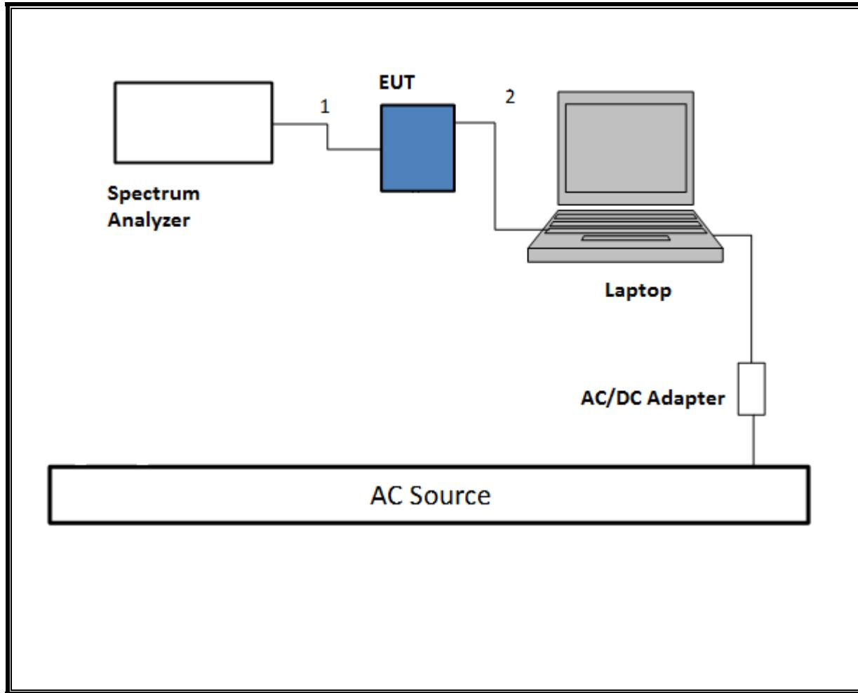
**TEST SETUP- RADIATED-ABOVE 1 GHZ**
