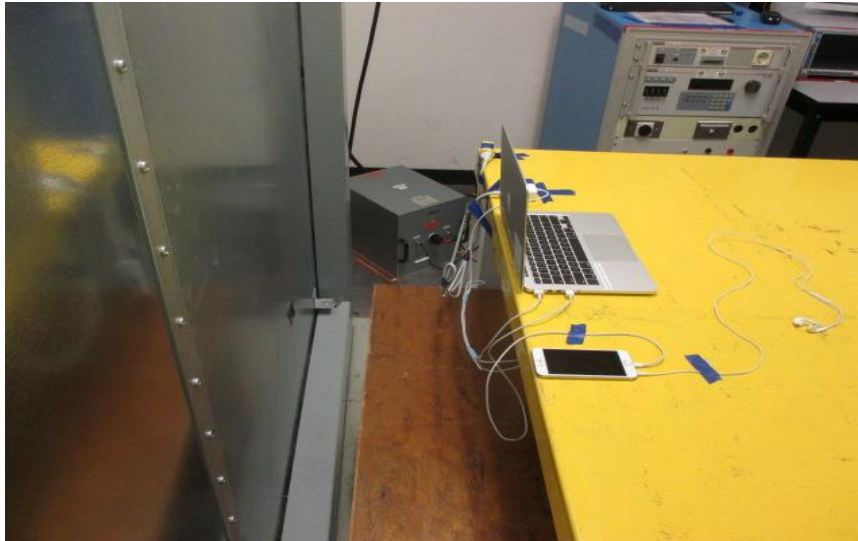
EUT WITH LAPTOP LINE CONDUCTED BACK PHOTO
