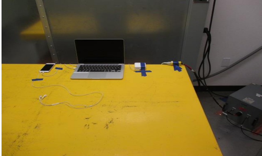
EUT WITH LAPTOP LINE CONDUCTED FRONT PHOTO
