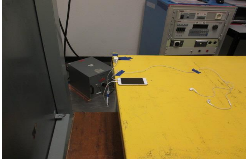
EUT ONLY LINE CONDUCTED BACK PHOTO
