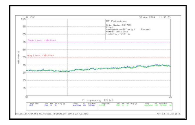
Note: GFSK, highest power mode used for test.
