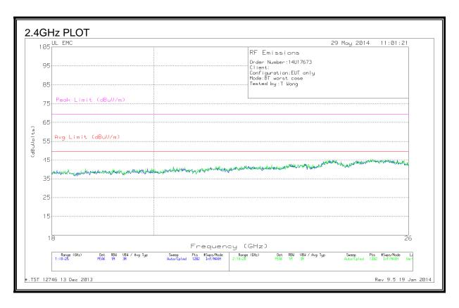
Note: GFSK, highest power mode used for test.
