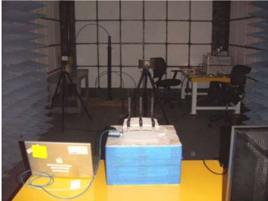
DFS BACK PHOTO (CLIENT-TO-CLIENT COMMUNICATIONS MODE SETUP)
