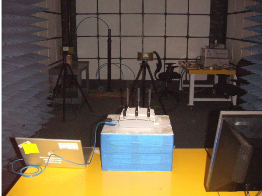
DFS FRONT PHOTO (CLIENT-TO-CLIENT COMMUNICATIONS MODE SETUP)
