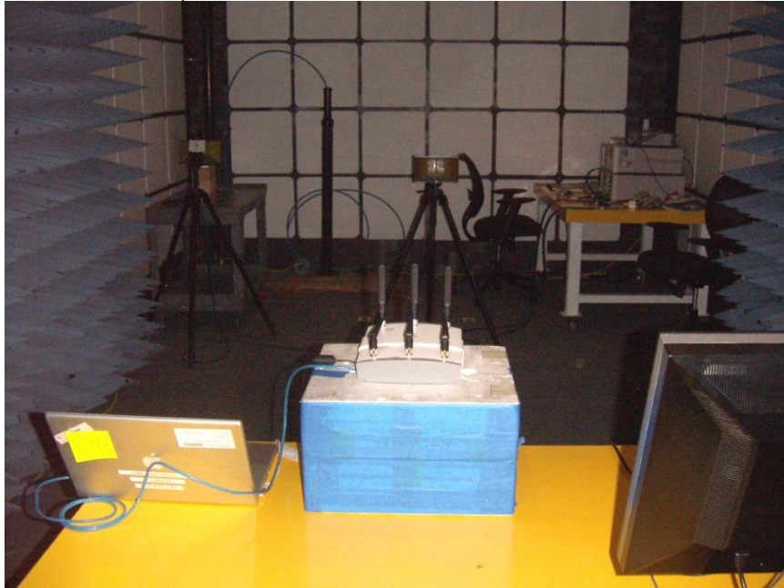
DFS FRONT PHOTO (CLIENT-TO-CLIENT COMMUNICATIONS MODE SETUP)
