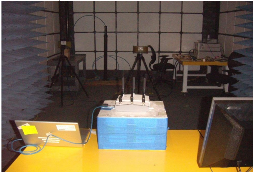
DFS FRONT PHOTO (CLIENT-TO-CLIENT COMMUNICATIONS MODE SETUP)
