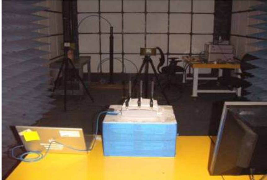
DFS FRONT PHOTO (CLIENT-TO-CLIENT COMMUNICATIONS MODE SETUP)
