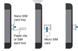
**Install the SIM card:** Insert the end of a small paper clip or SIM eject tool into the hole on the SIM card tray. Pull out the SIM card tray and place the SIM card in the tray as shown. With the tray aligned and the SIM card on top, carefully replace the tray.
