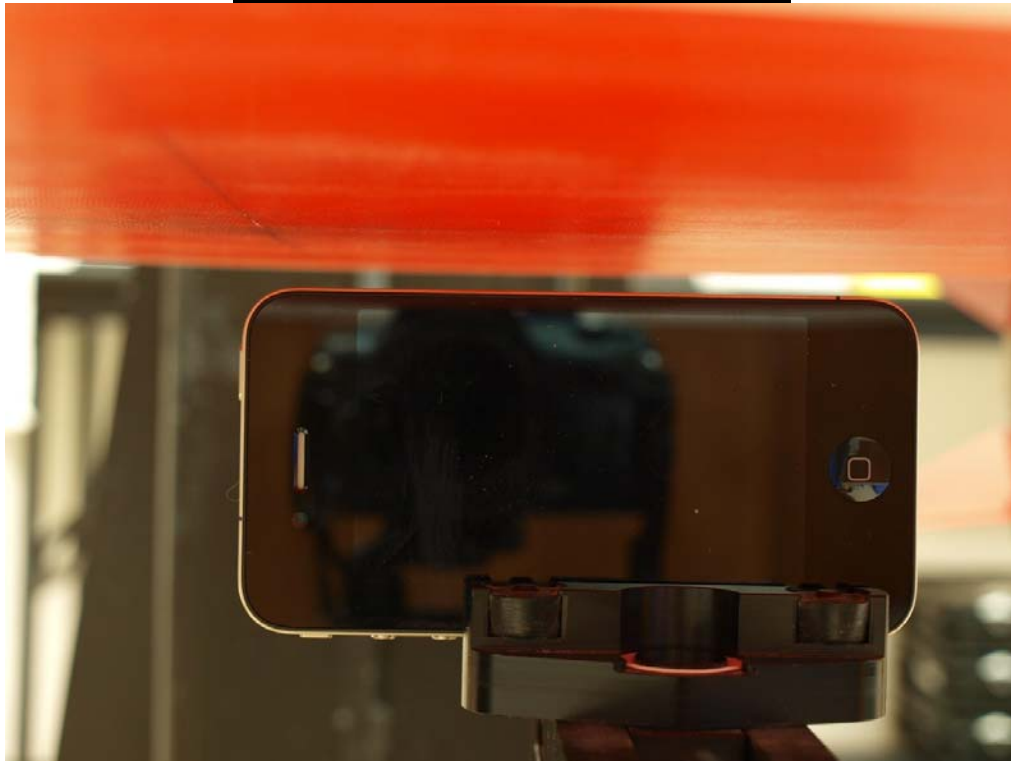
BODY – RIGHT EDGE w/ 1 cm Separation
