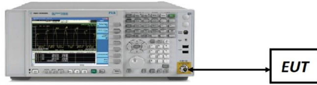
Figure 7-1. Test Instrument & Measurement Setup
