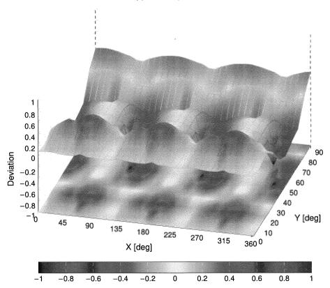
Probe isotropy for  $E_{tot}$ : probe rotated  $\phi=0^\circ$  to 360°, tilted from field propagation direction  $\vec{k}$  Parallel to the field propagation ( $\psi=0^\circ-90^\circ$ ) at 30 GHz: deviation within  $\pm 0.49$  dB Parallel to the field propagation ( $\psi=0^\circ-90^\circ$ ) at 60 GHz: deviation within  $\pm 0.55$  dB
