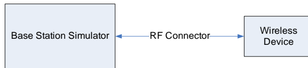
Figure 8-1 Power Measurement Setup
