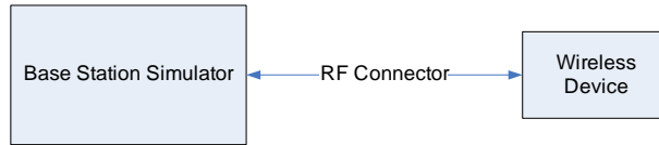
Figure 8-2 Power Measurement Setup
