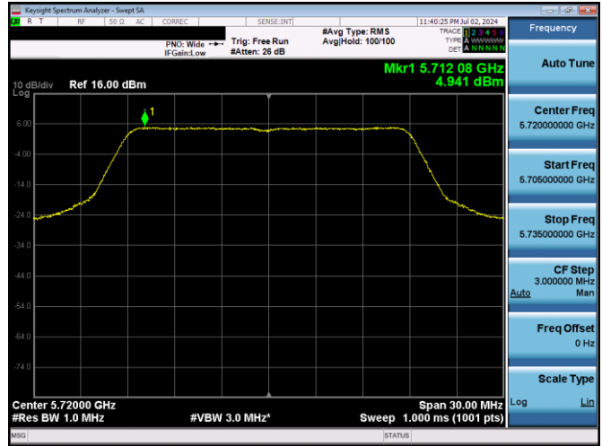
Plot 7-24. PSD (20MHz BW 802.11n - Ch. 144, MCS0)
