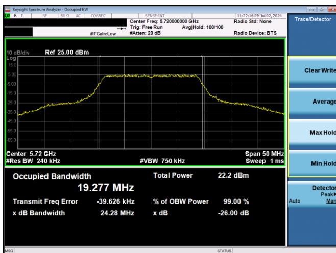
Plot 7-9. 26dB BW & 99% OBW (20MHz BW 802.11n – Ch. 144, MCS0)
