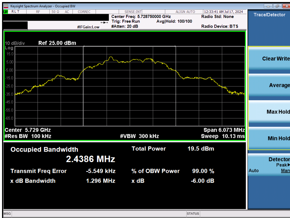
Plot 7-4. 6dB BW & 99% OBW (O-QPSK, 5728.75MHz, 500kbps)
