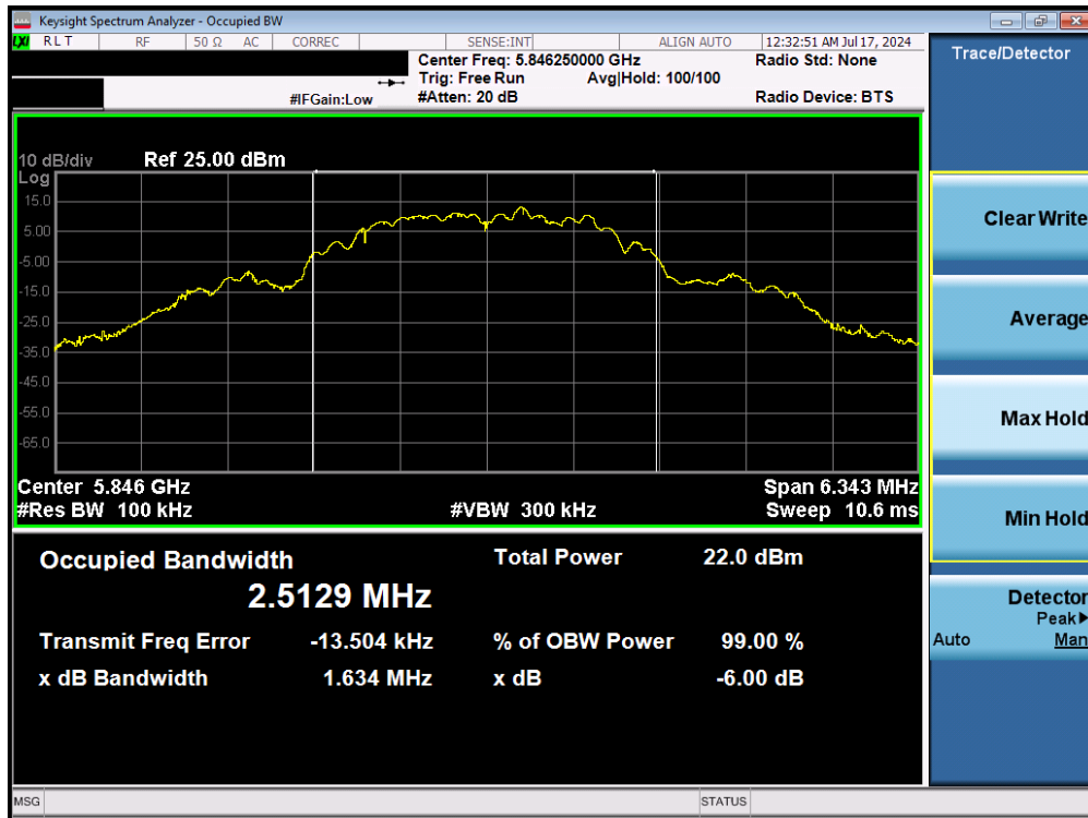
Plot 7-3. 6dB BW & 99% OBW (O-QPSK, 5846.25MHz, 250kbps)
