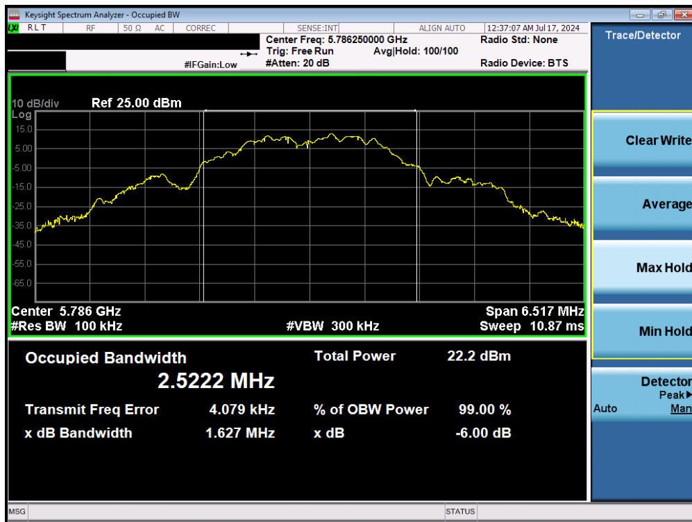
Plot 7-8. 6dB BW & 99% OBW (O-QPSK, 5786.25MHz, 1000kpbs)
