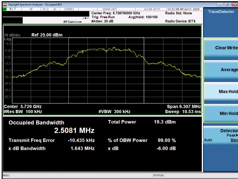
Plot 7-1. 6dB BW & 99% OBW (O-QPSK, 5728.75MHz, 250kbps)
