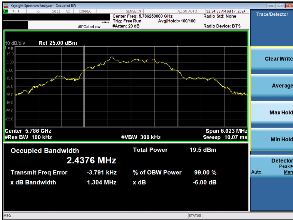
Plot 7-5. 6dB BW & 99% OBW (O-QPSK, 5786.25MHz, 500kbps)
