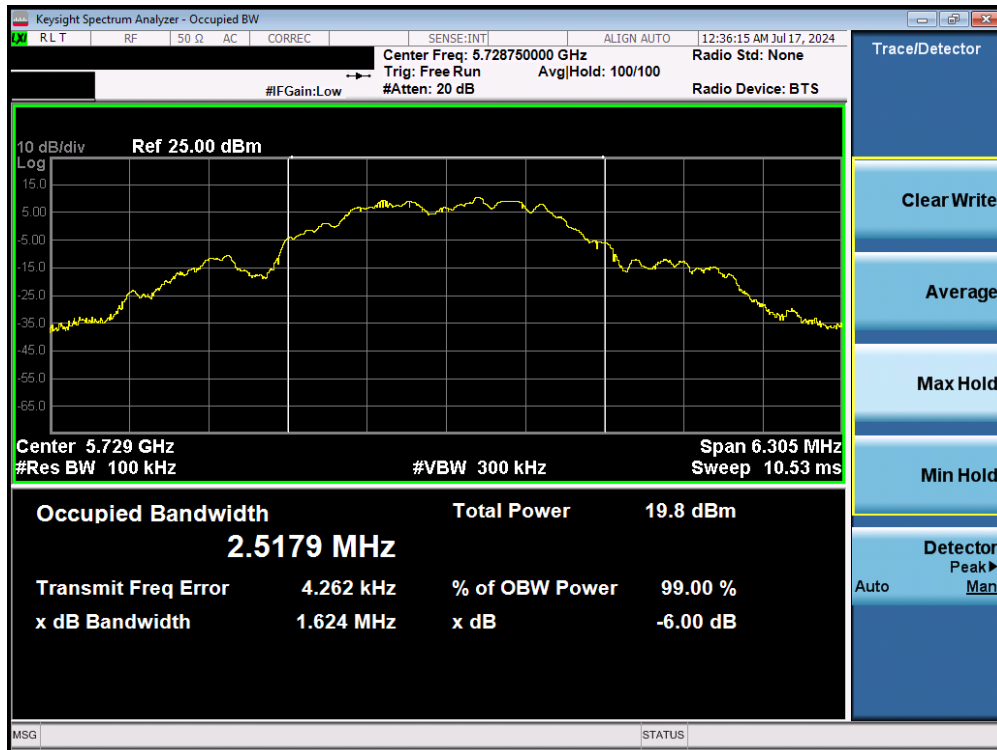
Plot 7-7. 6dB BW & 99% OBW (O-QPSK, 5728.75MHz, 1000kpbs)
