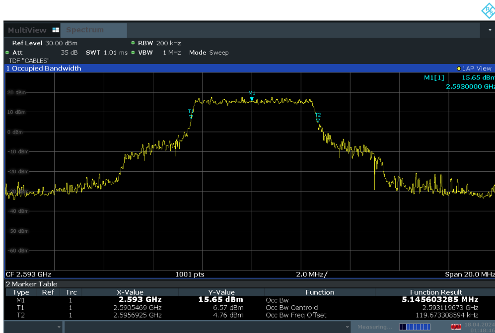
Plot 7-12. Occupied Bandwidth Plot (LTE Band 41 - 10MHz 16-QAM - Full RB)
