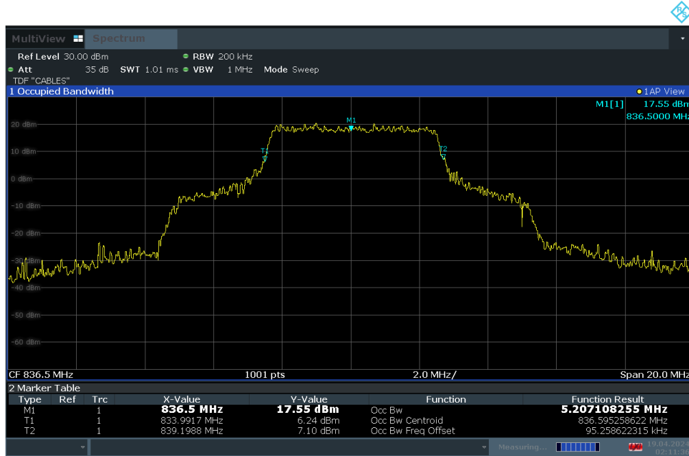
Plot 7-8. Occupied Bandwidth Plot (LTE Band 26/5 - 10MHz 16-QAM - Full RB Configuration)
