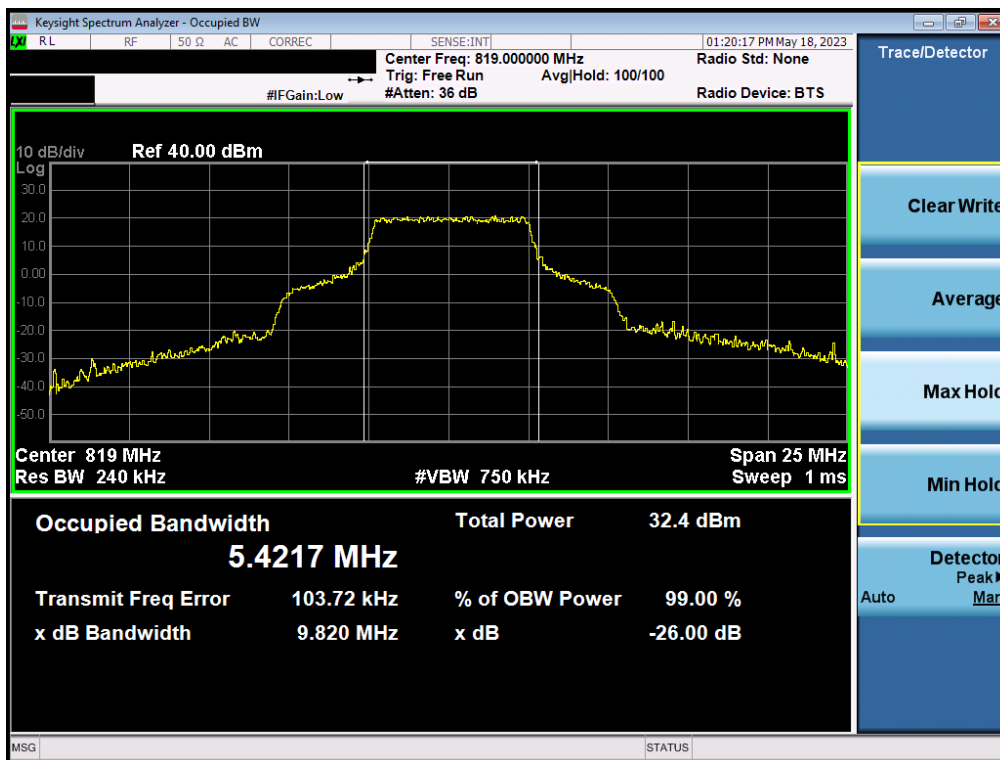
Plot 7-8. Occupied Bandwidth Plot (LTE Band 26 - 10MHz 16-QAM - Full RB Configuration)
