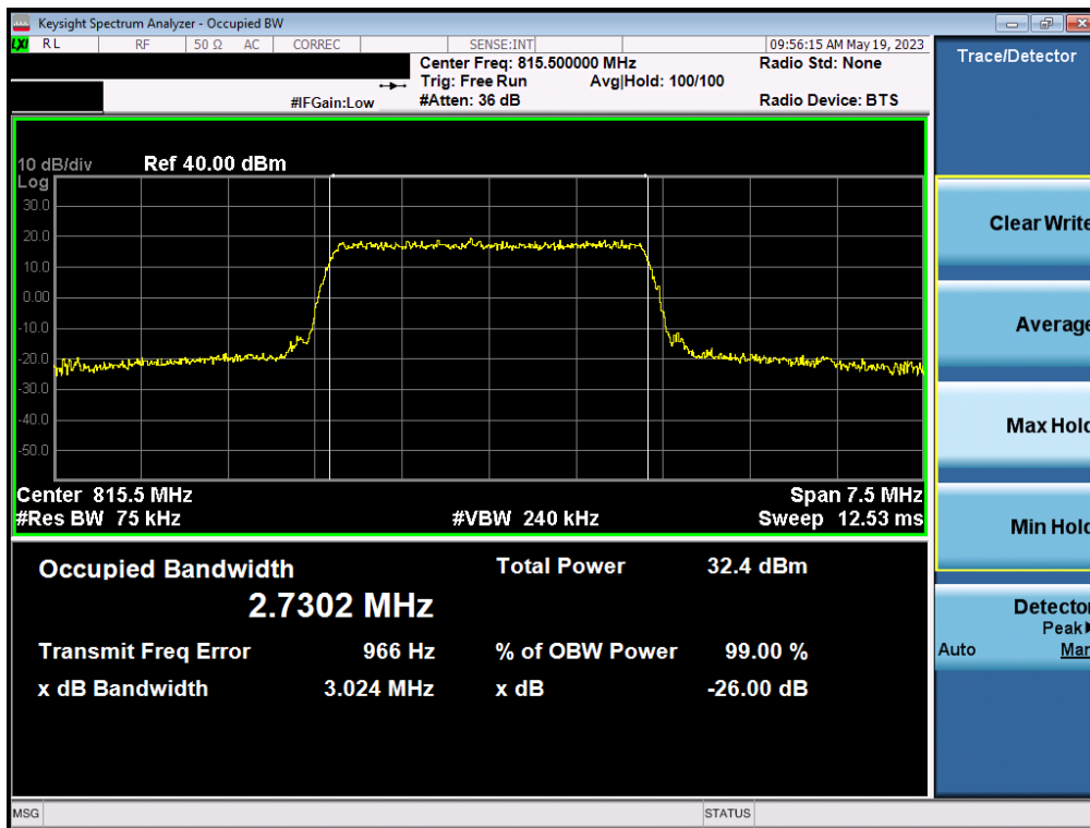
Plot 7-4. Occupied Bandwidth Plot (LTE Band 26 - 3MHz 16-QAM - Full RB Configuration)
