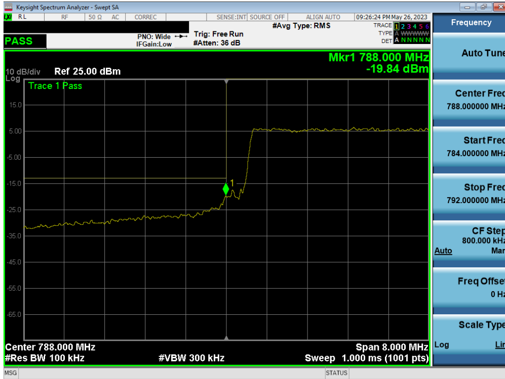
Plot 7-42. Lower Band Edge Plot (LTE Band 14, 10MHz QPSK - RB Size 50)
