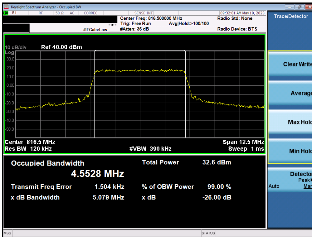
Plot 7-6. Occupied Bandwidth Plot (LTE Band 26 - 5MHz 16-QAM - Full RB Configuration)
