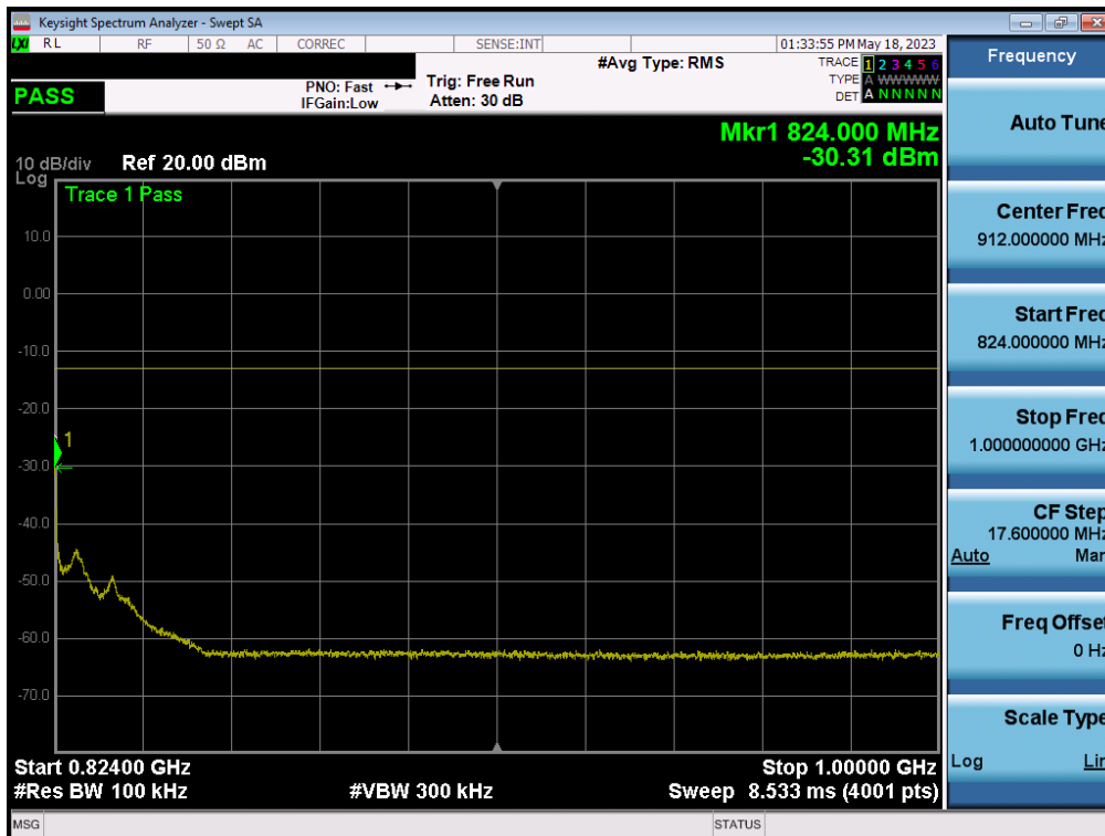
Plot 7-17. Conducted Spurious Plot (LTE Band 26 - 10MHz QPSK - RB Size 1, RB Offset 0 – Mid Channel)
