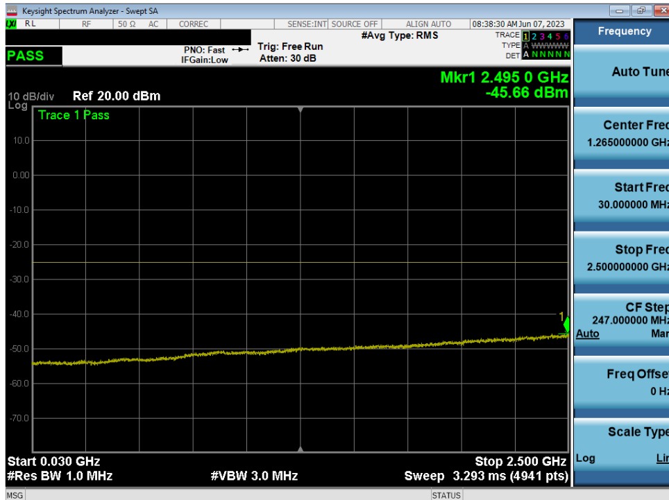
Plot 7-23. Conducted Spurious Plot (LTE Band 7 - 20MHz QPSK - RB Size 1, RB Offset 0 - High Channel)
