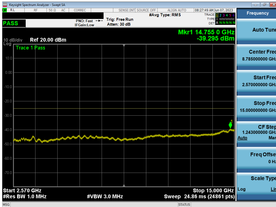
Plot 7-18. Conducted Spurious Plot (LTE Band 7 - 20MHz QPSK - RB Size 1, RB Offset 0 - Low Channel)
