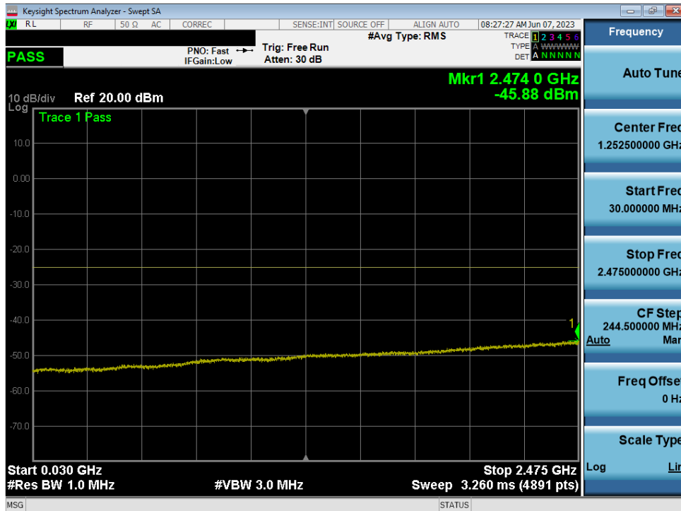
Plot 7-17. Conducted Spurious Plot (LTE Band 7 - 20MHz QPSK - RB Size 1, RB Offset 0 - Low Channel)
