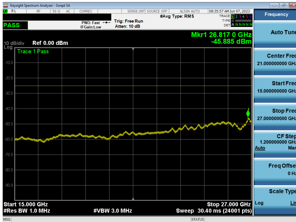
Plot 7-22. Conducted Spurious Plot (LTE Band 7 - 20MHz QPSK - RB Size 1, RB Offset 0 - Mid Channel)
