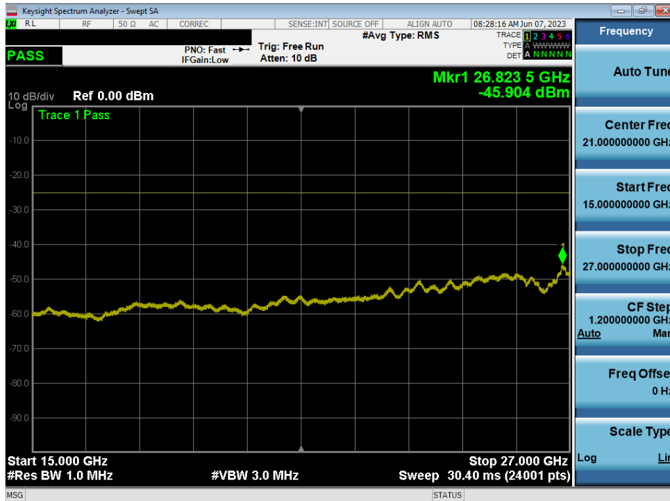
Plot 7-19. Conducted Spurious Plot (LTE Band 7 - 20MHz QPSK - RB Size 1, RB Offset 0 - Low Channel)
