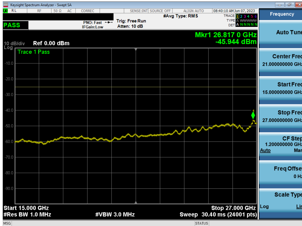
Plot 7-25. Conducted Spurious Plot (LTE Band 7 - 20MHz QPSK - RB Size 1, RB Offset 0 - High Channel)
