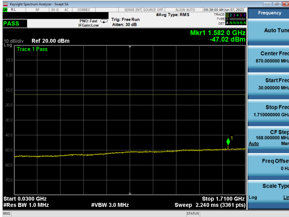
Plot 7-32. Conducted Spurious Plot (LTE Band 66/4 - 20MHz QPSK - RB Size 1, RB Offset 0 - High Channel)
