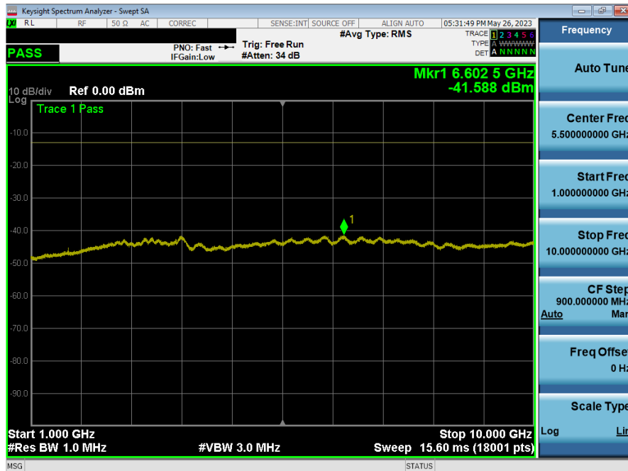
Plot 7-15. Conducted Spurious Plot (LTE Band 26/5 - 10MHz QPSK - RB Size 1, RB Offset 0 - Mid Channel)
