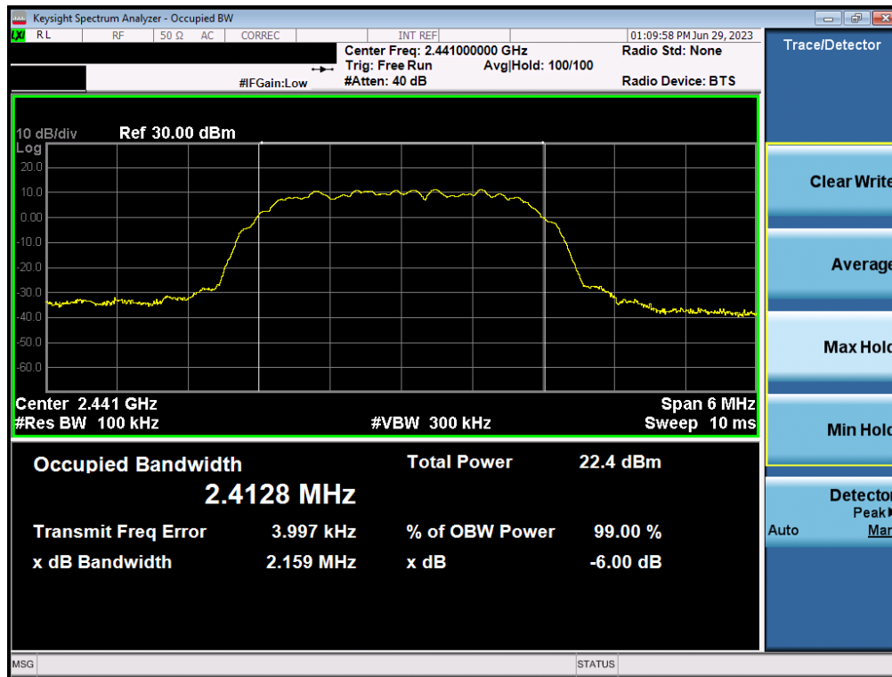
Plot 7-2. 6dB BW & 99% OBW Plot (Bluetooth (HDR4), 4Mbps, ePA – Ch. 38)
