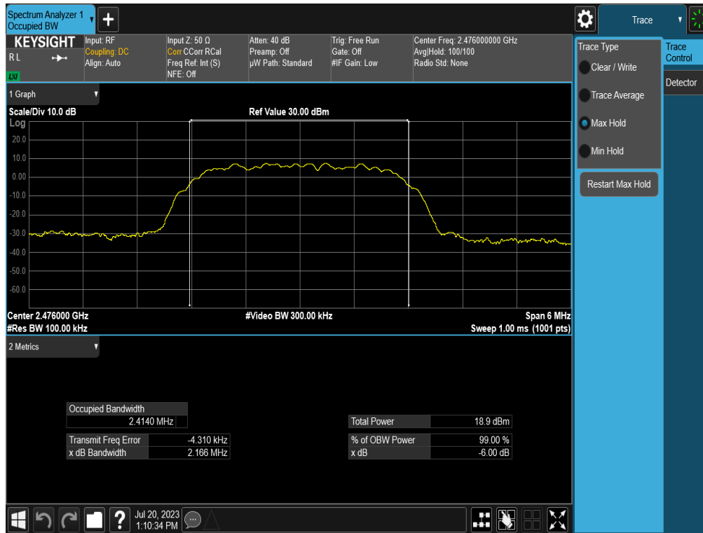
Plot 7-3. 6dB BW & 99% OBW Plot (Bluetooth (HDR4), 4Mbps, ePA – Ch. 73)
