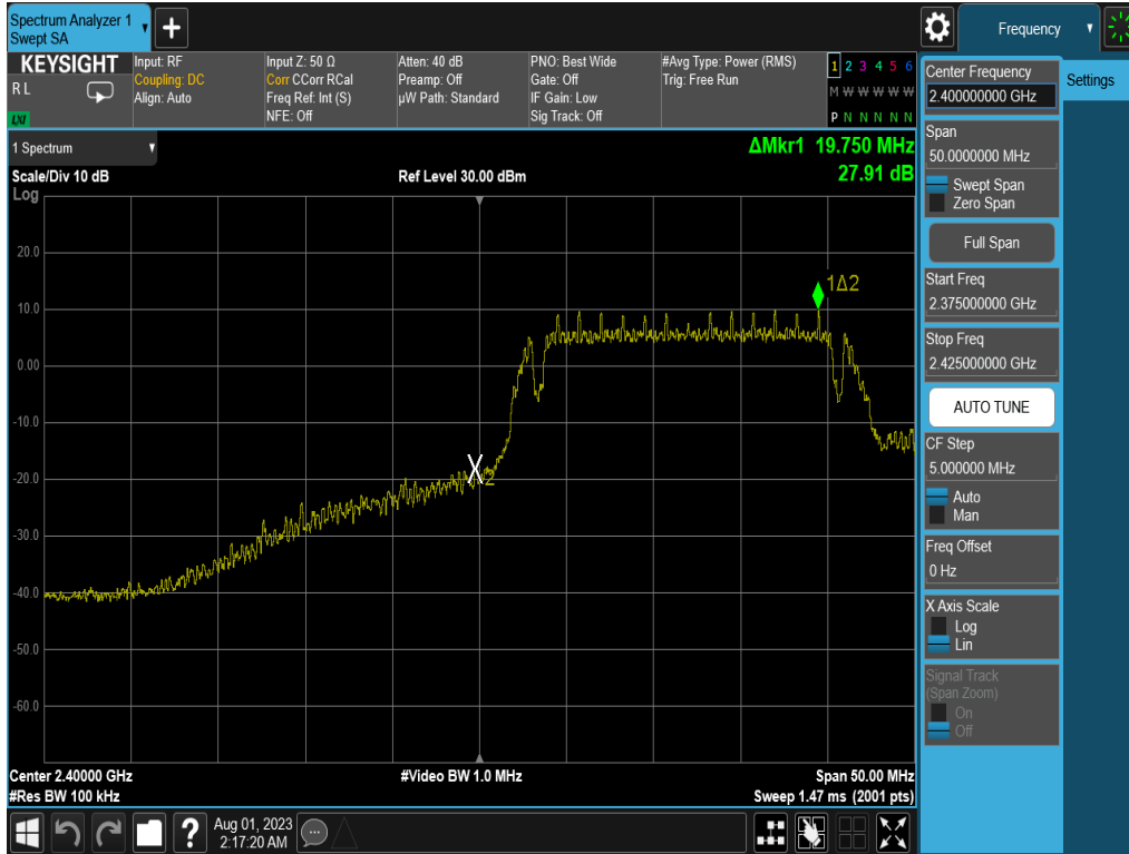
Plot 7-29. Band Edge Plot (802.11g- Ch. 1)
