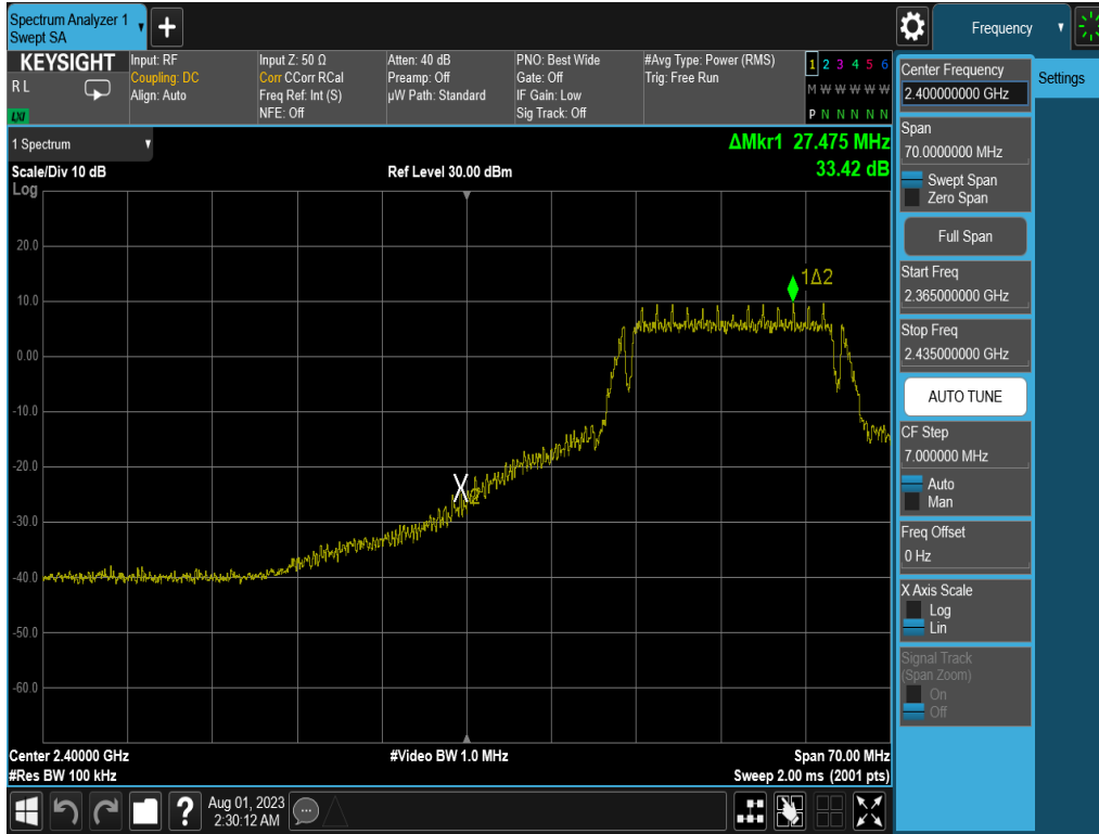
Plot 7-31. Band Edge Plot (802.11g– Ch. 3)
