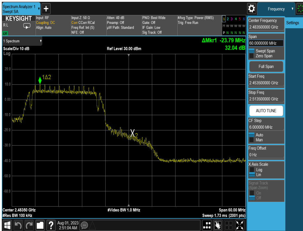
Plot 7-36. Band Edge Plot (802.11g – Ch. 13)
