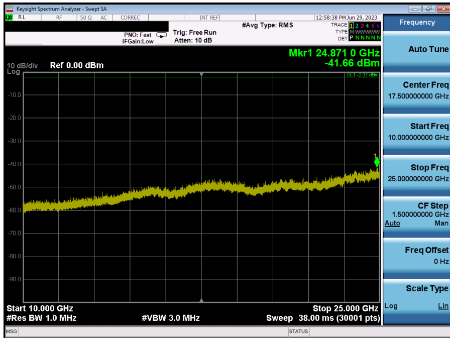
Plot 7-24. Conducted Spurious Plot (Bluetooth (LE), 1Mbps, ePA – Ch. 0)
