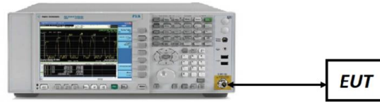
Figure 7-1. Test Instrument & Measurement Setup
