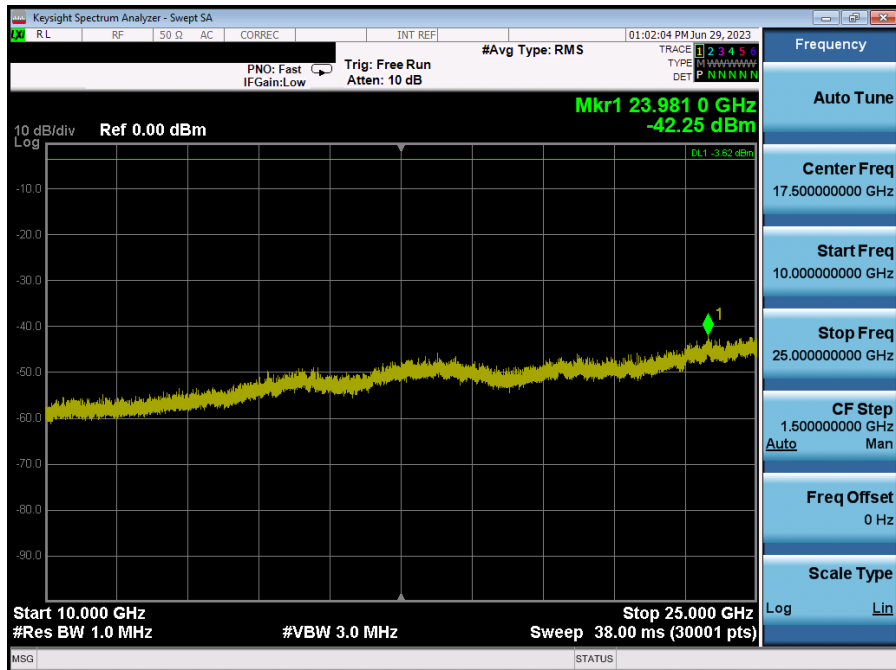
Plot 7-28. Conducted Spurious Plot (Bluetooth (LE), 1Mbps, ePA – Ch. 39)
