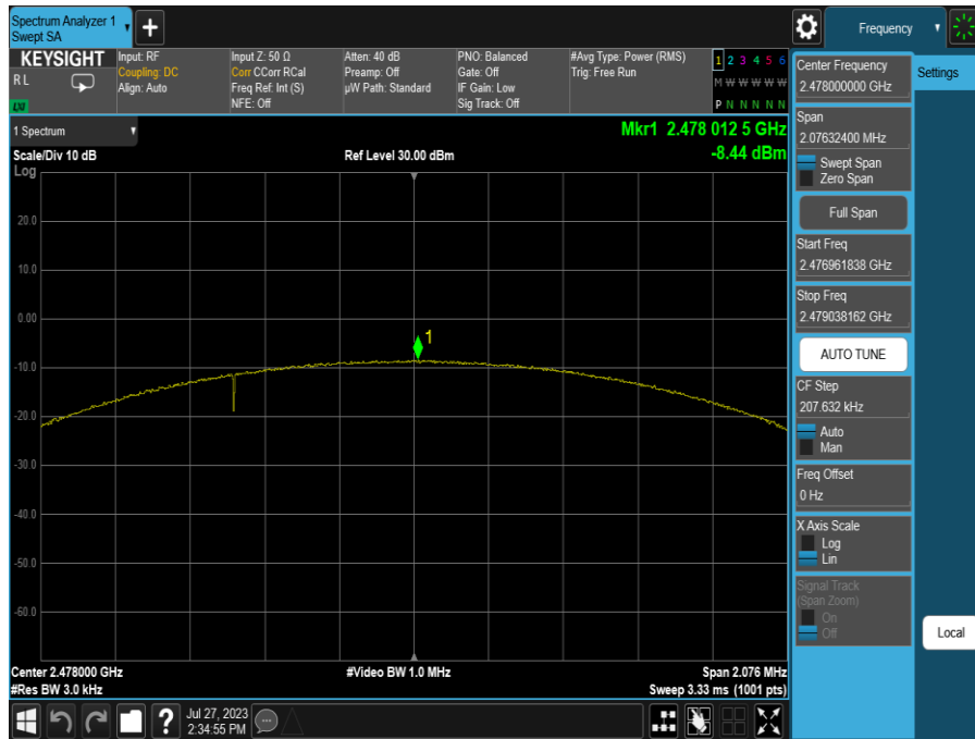
Plot 7-18. Power Spectral Density Plot (Bluetooth (LE), 2Mbps, iPA – Ch. 38)
