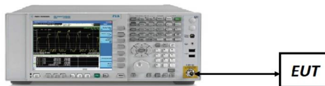
Figure 7-1. Test Instrument & Measurement Setup
